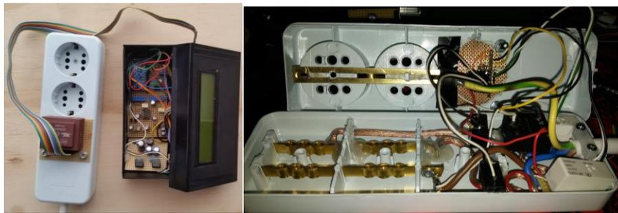
**Fig. 5** The image of Arduino module and the custom power plug
