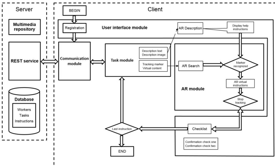
Fig. 2 Architecture of the system
