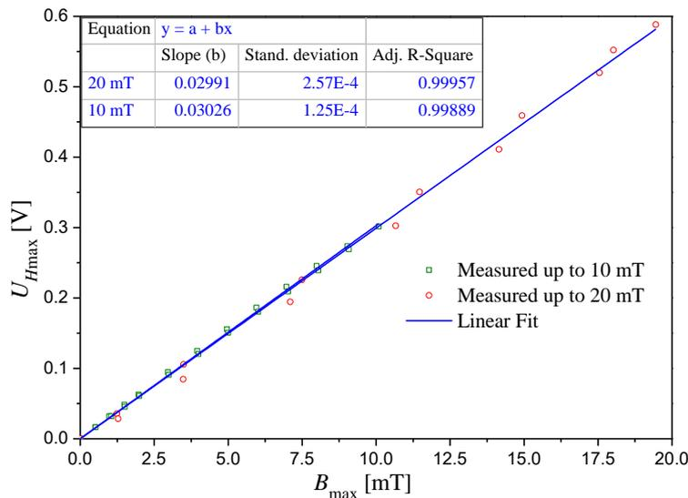
Fig. 5 Calibration of Hall sensor - measurement results and linear fit
