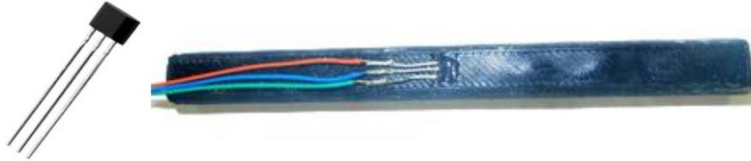
**Fig. 4** Hall sensor and its position inside plastic holder
