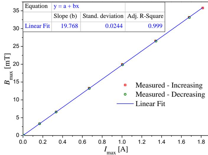
Fig. 6 Calibration of large solenoid - measurement results and linear fit
