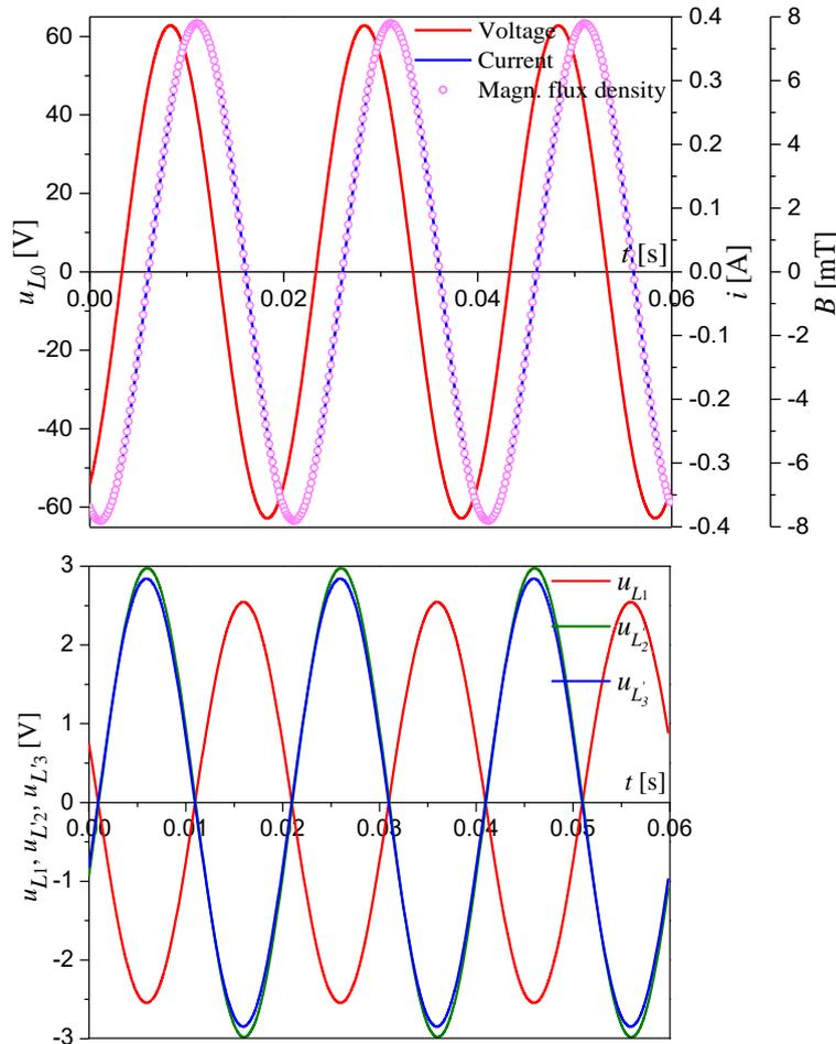
**Fig. 7** Calibration of pickup coils - measured signals
