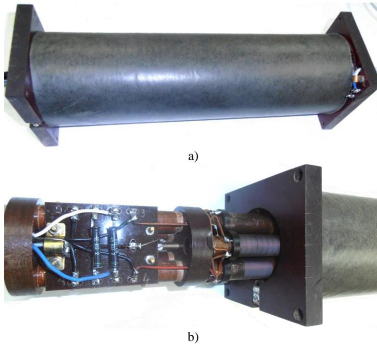
**Fig. 1** Photos of the induction magnetometer:
