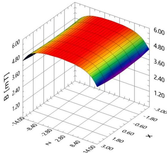
**Fig. 3** Total magnetic flux density distribution inside large solenoid
