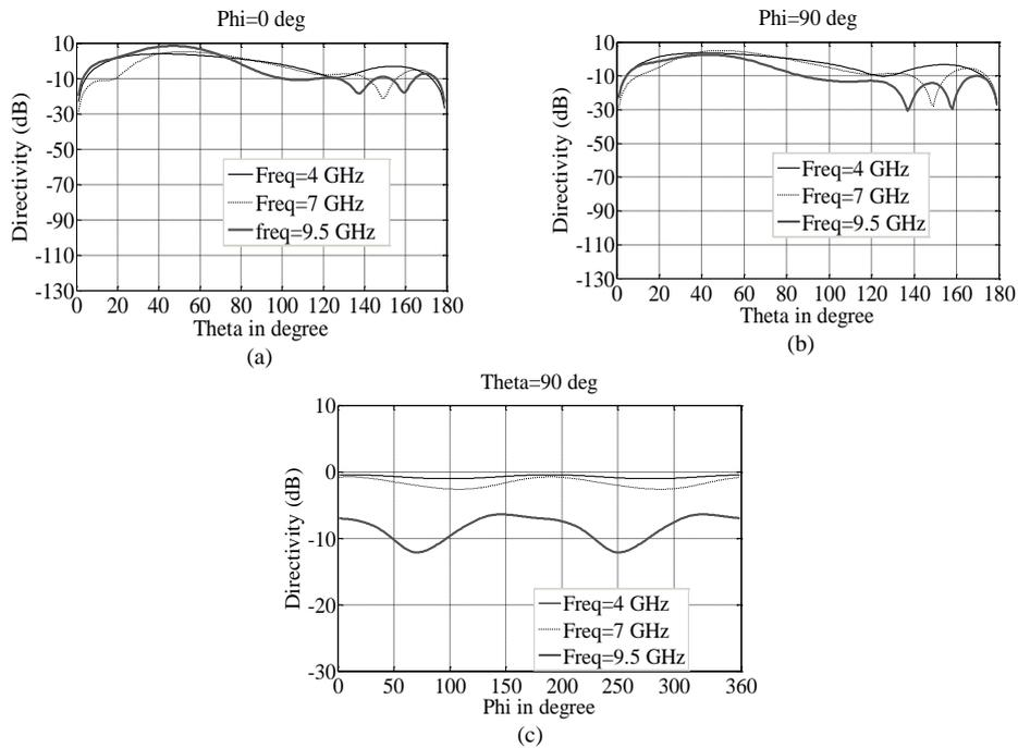
**Fig. 8** Radiation Pattern of monopole antenna with vertical crossed plates for three different frequencies for three sections with  $L1=15\text{mm}$ ,  $W1 = 18\text{mm}$ ,  $L2 = 7\text{mm}$ ,  $W2 = 8\text{mm}$ ,  $S = 5\text{mm}$ ,  $d=5\text{mm}$ ,  $g = 1.5\text{mm}$  and  $R = 50\text{mm}$ . (a)  $\Phi = 0^\circ$ , (b)  $\Phi = 90^\circ$ , and (c)  $\Theta = 90^\circ$
