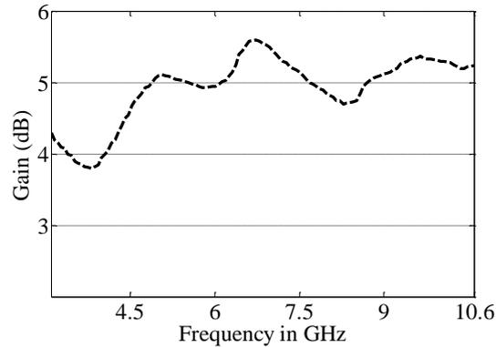
**Fig. 7** The vertical cross-sections monopole antenna gain with  $L1 = 15\text{mm}$ ,  $W1 = 18\text{mm}$ ,  $L2=7\text{mm}$ ,  $W2 = 8\text{mm}$ ,  $S = 5\text{mm}$ ,  $d = 5\text{mm}$ ,  $g = 1.5\text{mm}$  and  $R = 50\text{mm}$
