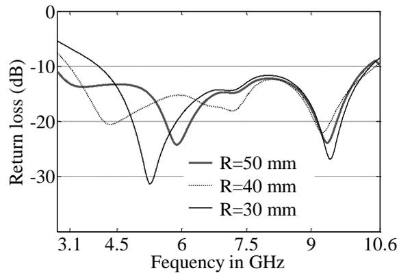
**Fig. 5** Antenna return loss for different radius  $R$  of circular ground plane with  $L_1 = 15\text{mm}$ ,  $W_1 = 18\text{mm}$ ,  $L_2 = 7\text{mm}$ ,  $W_2 = 8\text{mm}$ ,  $S = 5\text{mm}$ ,  $d = 5\text{mm}$  and  $g = 1.5\text{mm}$
