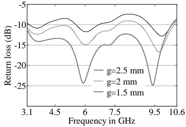
**Fig. 4** Antenna return loss for different heights  $g$  with  $L_1=15\text{mm}$ ,  $W_1 = 18\text{mm}$ ,  $L_2 = 7\text{mm}$ ,  $W_2 = 8\text{mm}$ ,  $S = 5\text{mm}$ ,  $d=5\text{mm}$  and  $R = 50\text{mm}$ .
