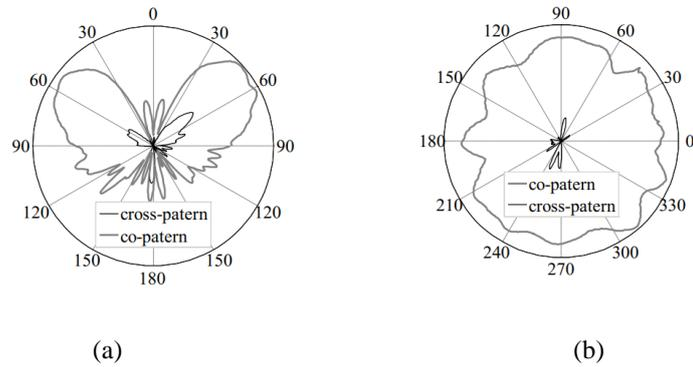
**Fig. 9** Measurement of co and cross-radiation patterns of proposed structure at 4 GHz (a) E-plane (xz-plane) and (b) H-plane (xy-plane.  $L_1=15\text{mm}$ ,  $W_1 = 18\text{mm}$ ,  $L_2 = 7\text{mm}$ ,  $W_2 = 8\text{mm}$ ,  $S = 5\text{mm}$ ,  $d=5\text{mm}$ ,  $g = 1.5\text{mm}$  and  $R = 50\text{mm}$ .)
