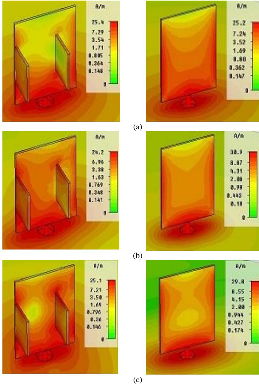
**Fig. 6** Comparison of current distribution ( $A/m$ ) for three frequencies.
