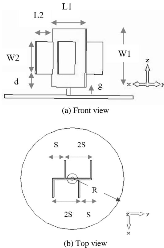
**Fig. 1** A monopole antenna including vertical plates
