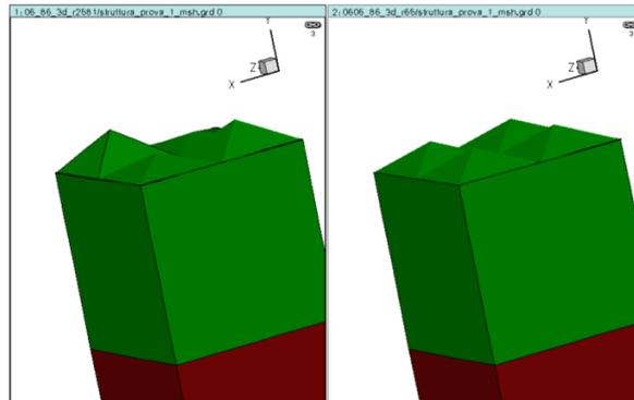
**Fig. 5** Senterus structure with non uniform (left) and uniform (right) pyramids
