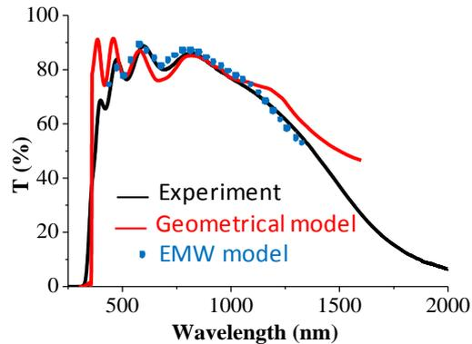
**Fig. 8** Measured and numerical transmittance profiles for a surface encountering diffraction effects. The EMW model correctly reproduces the experimental curve.
