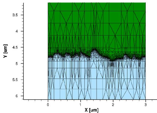
**Fig. 3** Sentaurus 2D mesh for the cross section of an AFM image
