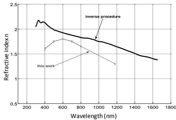
**Fig. 15** Comparison between the real part of the refractive index for a ZnO on glass thin layer measured by means of an ellipsometric method (inverse procedure) and the one achieved in this work
