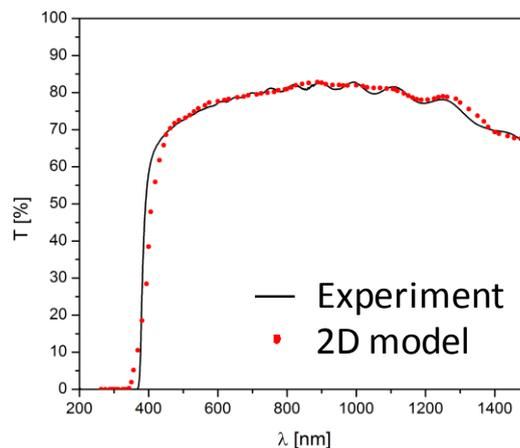
**Fig. 7** Comparison between a measured transmittance and a numerical result achieved by means of the ray-tracing model.
