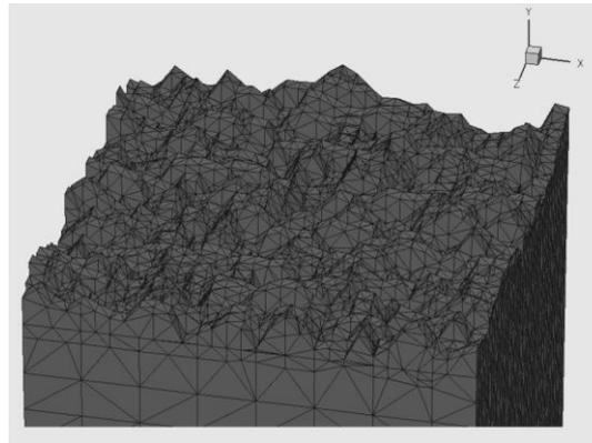
**Fig. 4** Three dimensional Sentaurus mesh for an AFM image
