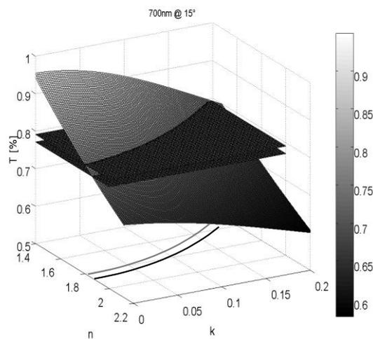
**Fig. 12** Transmittance surface and measured transmittance for a 15° incidence angle.
