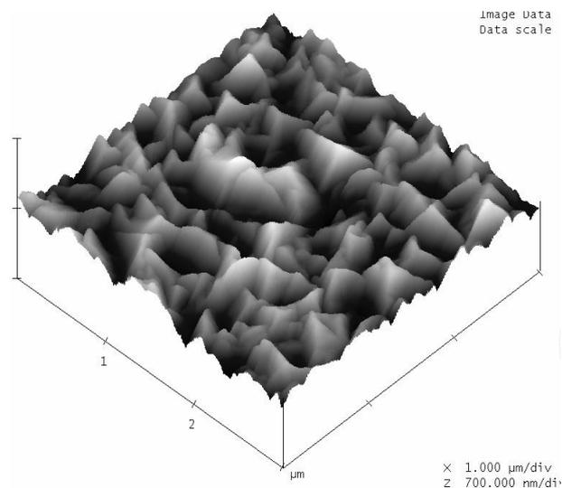
**Fig. 1** AFM image of a CVD deposited ZnO thin film
