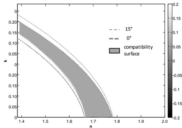
**Fig. 13** Locus of refractive index giving the transmittance measured for both  $0^\circ$  and  $15^\circ$  incidence angle.
