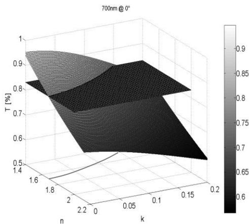
**Fig. 10** Intercept between the transmittance surface and the measured transmittance. The line is the locus of all refractive indexes giving the same transmittance for the assigned ZnO on glass structure.
