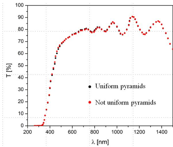
**Fig. 6** Transmittances profiles evaluated by Senterus for structures with different surface shape but same effective roughness.
