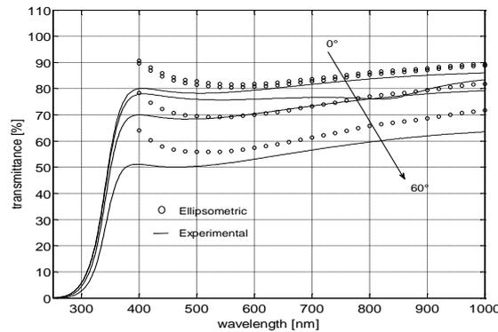
**Fig. 16** Comparison between measured transmittance profiles and the transmittance profiles evaluated by Sentaurus when the refractive index measured by means of the ellipsometric procedure were used.
