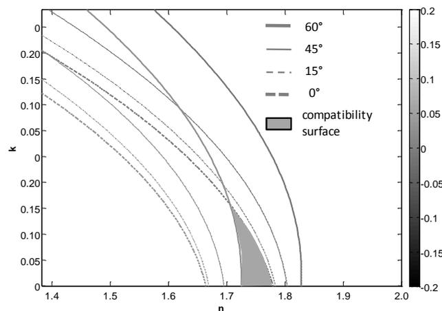
**Fig. 14** Locus of refractive index giving the transmittance measured for  $0^\circ$ ,  $15^\circ$ ,  $45^\circ$ ,  $60^\circ$  incidence angle.
