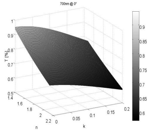
**Fig. 9** Transmittance for a ZnO on glass structure as a function of the complex refractive index of the ZnO
