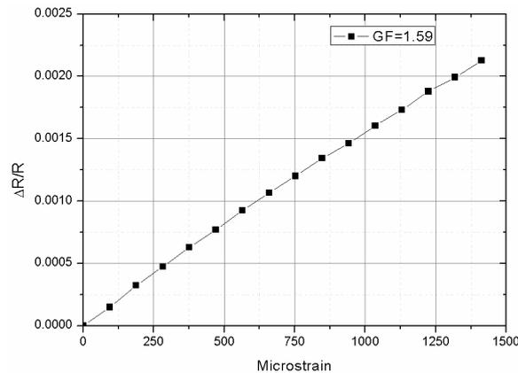
**Fig. 9** Relative resistance change  $\Delta R/R$  as a function of the applied microstrain for compressive strain for second series of tested strain gages.
