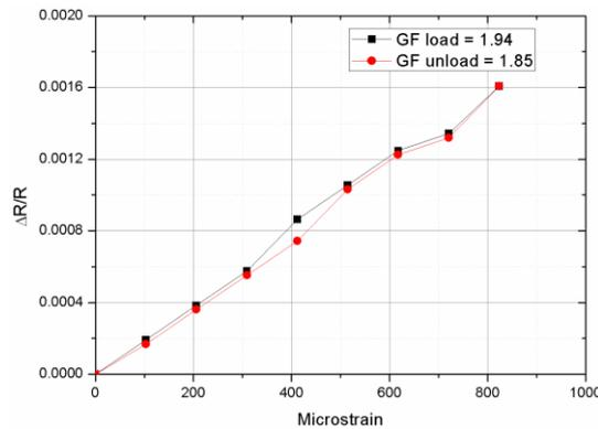
**Fig. 11** Relative resistance change  $\Delta R/R$  as a function of the applied mechanical deformation for third series of tested strain gages (one printed layer).
