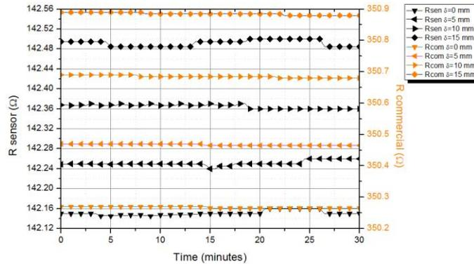
**Fig. 10** Time response of one sample strain gage from second series of tested gages (denoted *R<sub>sensor</sub>*) and commercial sensor CEA-06-125UN-350 by Micro-Measurements (denoted *R<sub>commercial</sub>*) under constant deflection of the steel beam.
