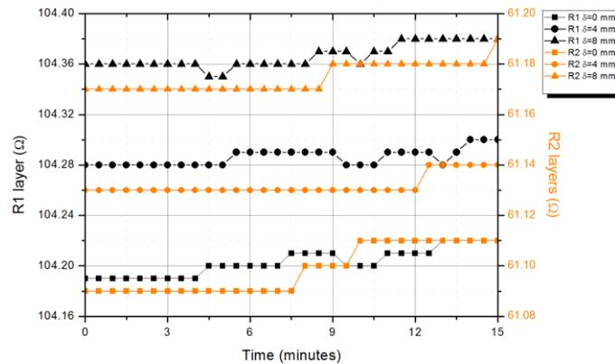
**Fig. 13** Time response under constant deflection of the steel beam for one printed layer ( $R1$  layer) and two printed layers ( $R2$  layers) strain gages.
