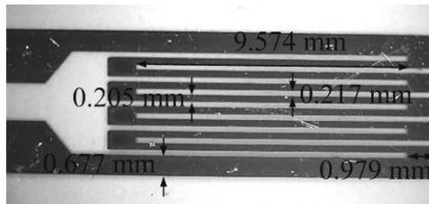
**Fig. 1** Representative sample of strain gages with geometrical dimensions
