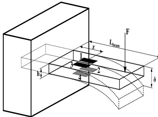
**Fig. 5** Cantilever with four placed strain gages (1, 2, 3 and 4) connected in a full-bridge Wheatstone circuit.
