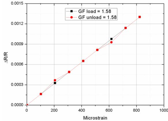
**Fig. 12** Relative resistance change  $\Delta R/R$  as a function of the applied mechanical deformation for third series of tested strain gages (two printed layers).
