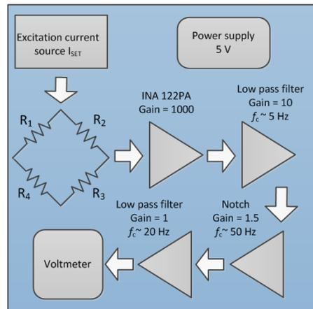
**Fig. 6** Block diagram of the developed signal conditioning circuit.
