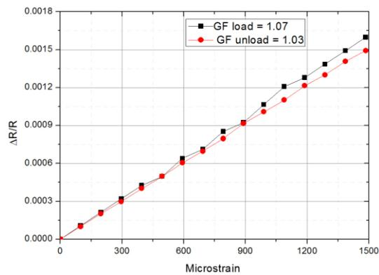
**Fig. 7** Relative resistance change  $\Delta R/R$  as a function of the applied microstrain for first series of printed strain gages for the loading (black line) and unloading (red line) of the beam.
