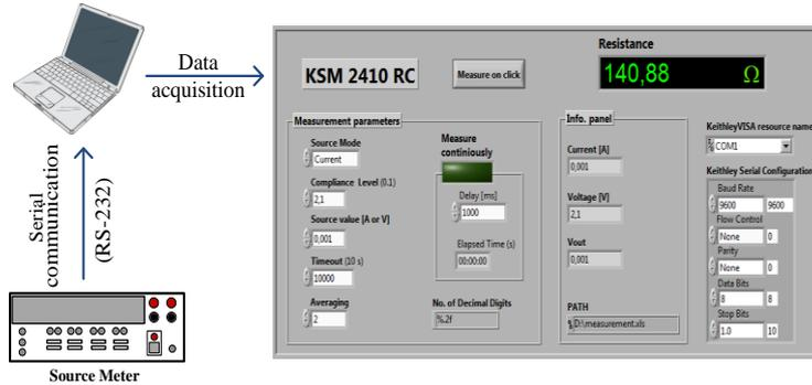
**Fig. 3** Principle of data acquisition using Keithley Source Meter 2410 and control software tool.
