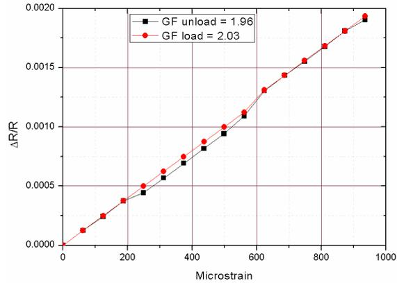
**Fig. 8** Relative resistance change  $\Delta R/R$  as a function of the applied microstrain for second series of printed strain gages for the loading (red line) and unloading (black line) of the beam.
