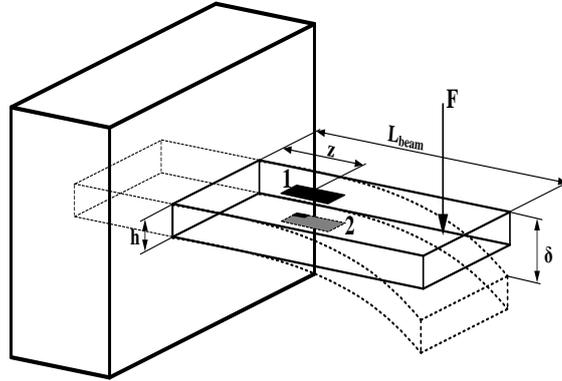
**Fig. 2** Gages placement for measuring tensile (gage denoted with “1”) and compressive (gage denoted with “2”) strain.
