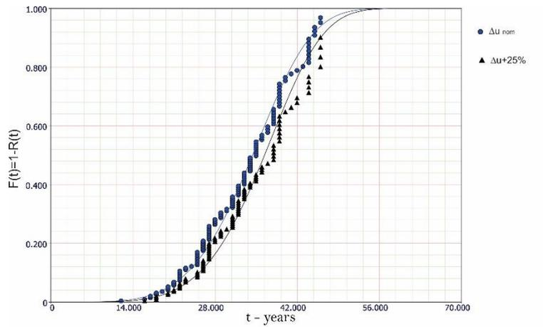
**Fig. 2** Weibull unreliability distribution for CBs on overhead feeders
