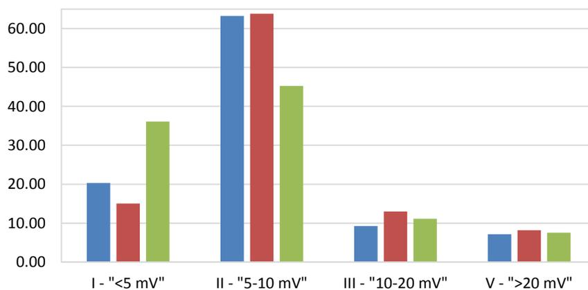
**Fig. 1** Voltage drop distribution on analyzed circuit breakers
