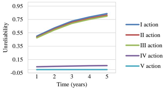
**Fig. 9** Power stations unreliability in next years for each action (Columns from table 3)
