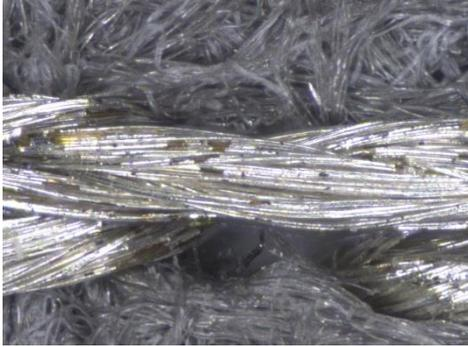
**Fig. 24** Failure mode of embroidered yarn on non-woven textile after cyclic bending. Damage to the Ag-coating of the filaments is visible.
