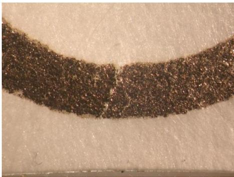
**Fig. 22** Failure mode of SPB-sample after test to 5% stretching [5]. Cracks are visible in the screen-printed layer.
