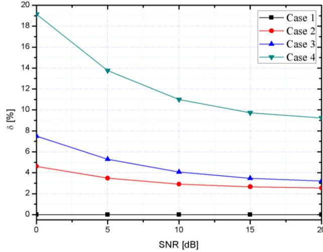
**Fig. 3** Relative difference in the symbol error probabilities of the ML and MAP detectors.
