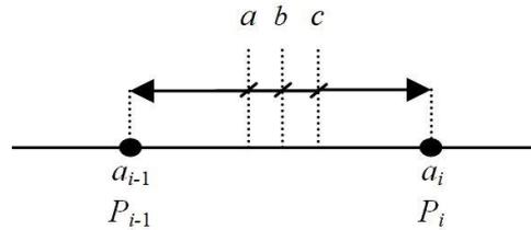
**Fig. 1** The decision thresholds for: 1) MAP detector  $m_i = a$  for  $P_{i-1} < P_i$ ,  $m_i = b$  for  $P_{i-1} = P_i$ ,  $m_i = c$  for  $P_{i-1} > P_i$ ; 2) ML detector  $m_i = b$ .
