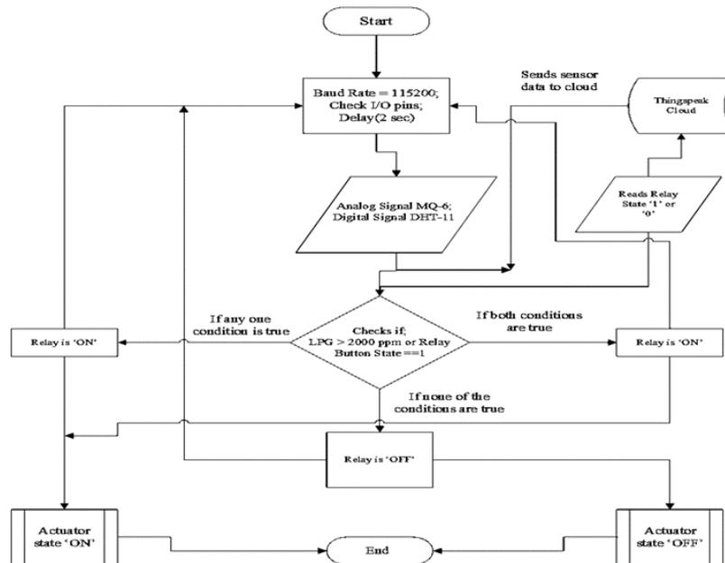
**Fig. 1** Flowchart of the fabricated control system.
