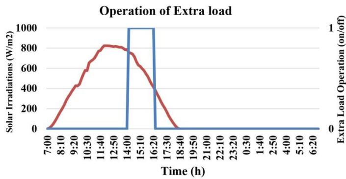
**Fig. 11** Extra load operation during the 24 hour time
