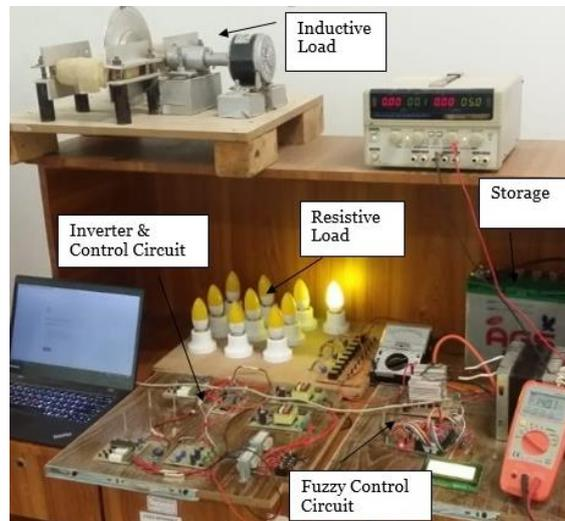
**Fig. 7** Microgrid testbed
