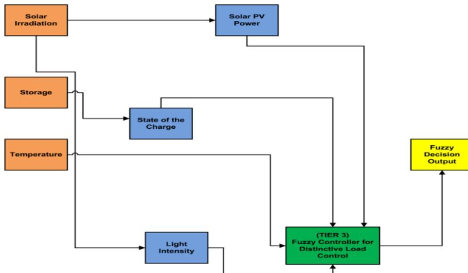
**Fig. 1** Proposed microgrid algorithm block diagram
