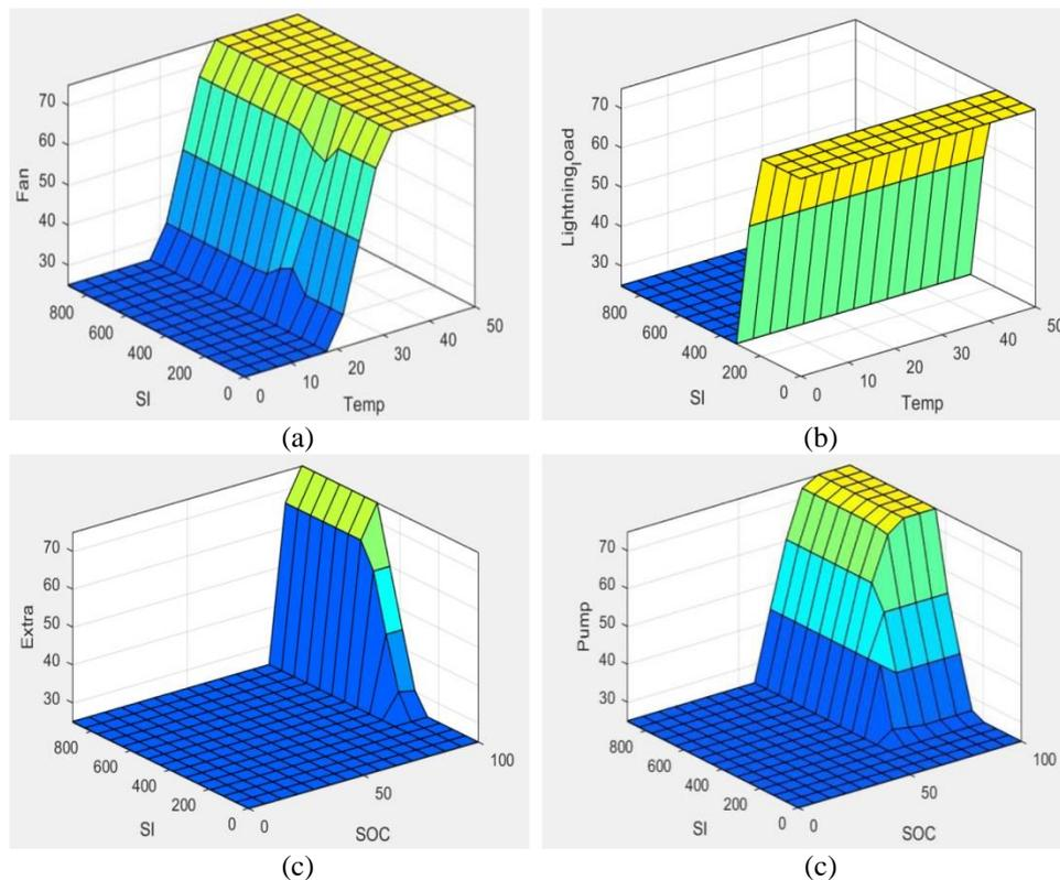
**Fig. 6** Fuzzy surface plots of the loads operation in response to the variation in the membership functions (a) shows the surface plot of fans (b) shows the surface plot of lights (c) shows the surface plot of extra load and (d) shows the surface plot of water pump
