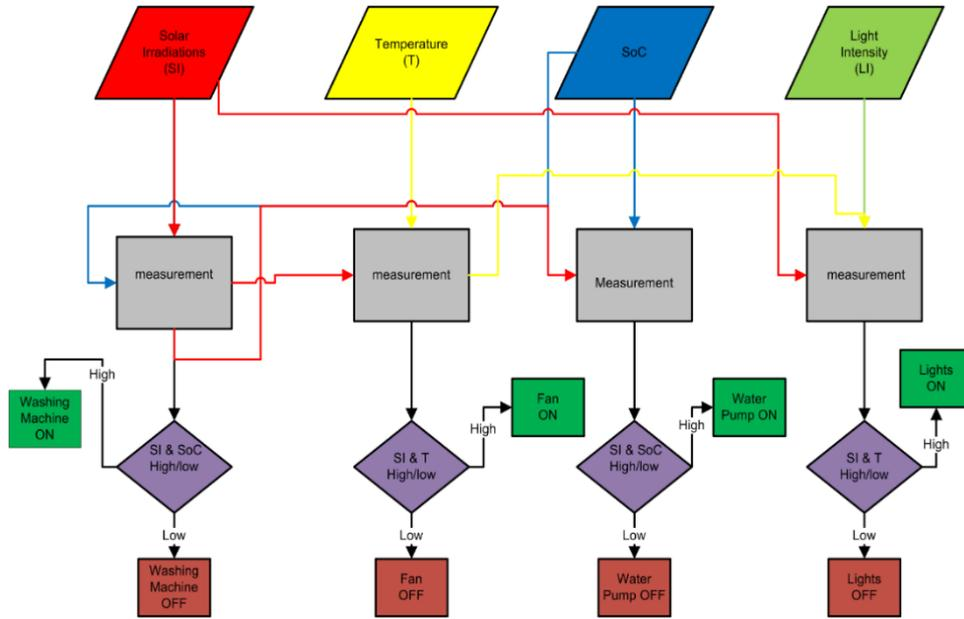
Fig. 2 Distinctive load controller flow diagram
