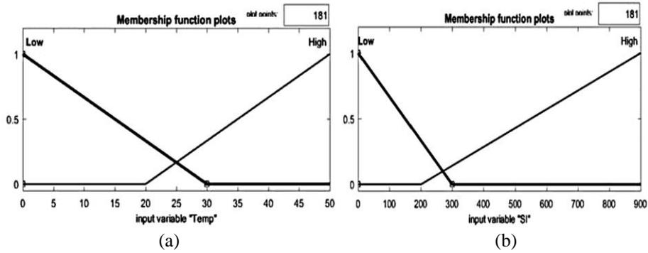
Fig. 3 Input membership function of Solar Irradiations for Fans and Lights
