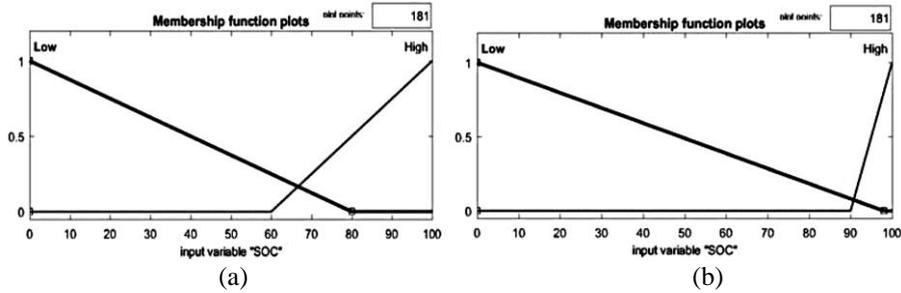
Fig. 4 (a) shows the input membership function of SoC for solar pump while (b) shows the input membership function SoC for extra load
