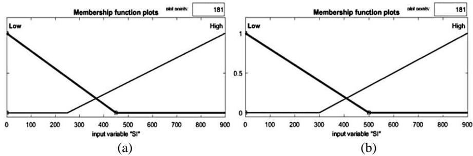
Fig. 5 (a) shows the input membership function of SI for extra load while (b) shows the input membership function SI for water pump
