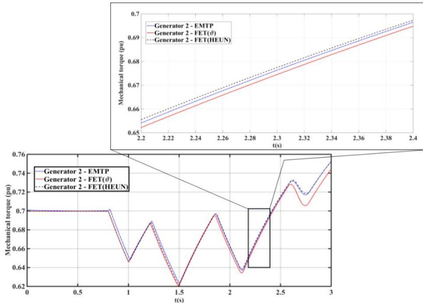
Fig. 5 Generator '2' mechanical power ( $P_m$ ) during angle stability simulation
