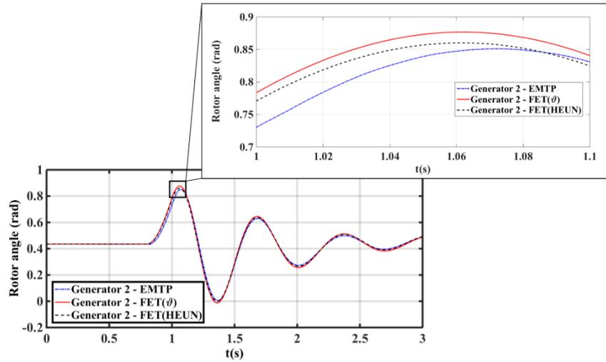
Fig. 3 Generator '2' rotor angle ( $\delta$ ) during angle stability simulation
