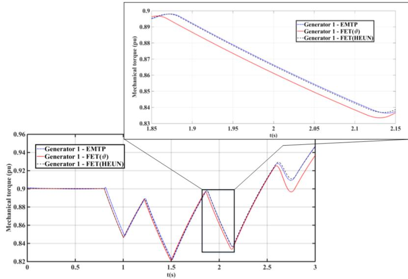
Fig. 4 Generator '1' mechanical power ( $P_m$ ) during angle stability simulation
