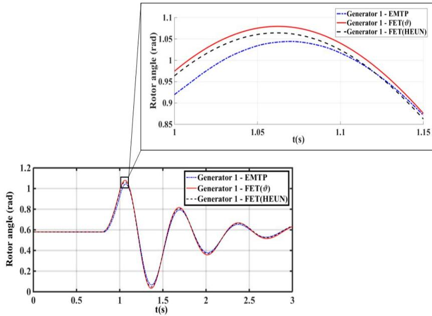
Fig. 2 Generator '1' rotor angle ( $\delta$ ) during angle stability simulation
