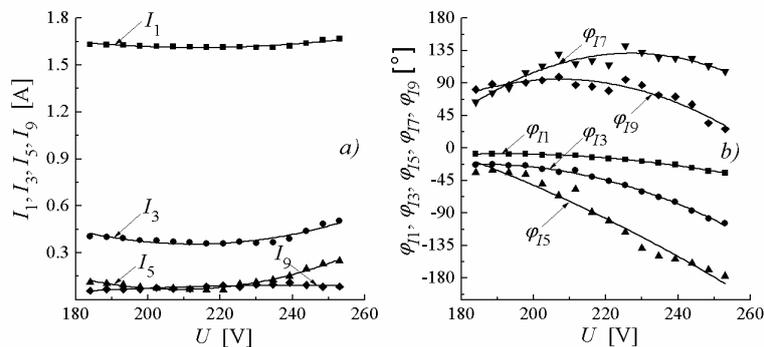
**Fig. 3** Measured values and corresponding fitting curves of: a) amplitudes of  $I_1$ ,  $I_3$ ,  $I_5$  and  $I_9$ , and b) angles of  $I_1$ ,  $I_3$ ,  $I_5$ ,  $I_7$ , and  $I_9$ , of air-conditioner
