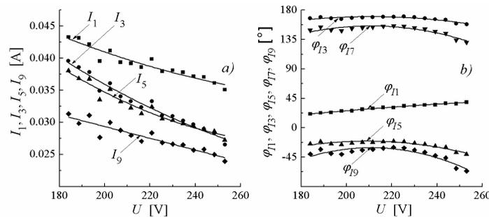
**Fig. 2** Measured values and corresponding fitting curves of: a) amplitudes of  $I_1$ ,  $I_3$ ,  $I_5$  and  $I_9$ , and b) angles of  $I_1$ ,  $I_3$ ,  $I_5$ ,  $I_7$ , and  $I_9$ , of laptop computer
