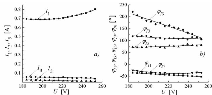
**Fig. 4** Measured values and corresponding fitting curves of: a) amplitudes of  $I_1$ ,  $I_3$  and  $I_5$ , and b) angles of  $I_1$ ,  $I_3$ ,  $I_5$ ,  $I_7$ , and  $I_9$ , of refrigerator
