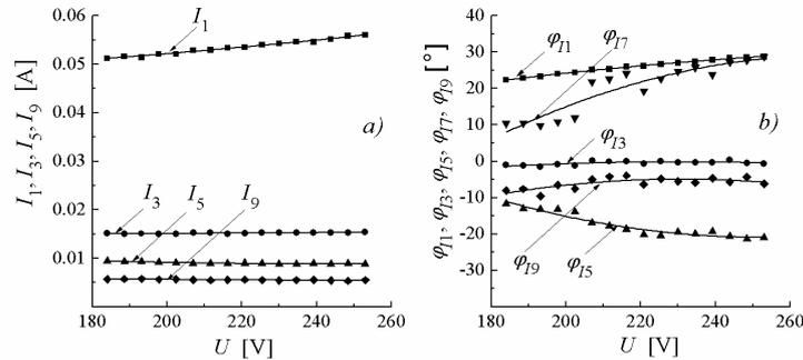
**Fig. 1** Measured values and corresponding fitting curves of: a) amplitudes of  $I_1$ ,  $I_3$ ,  $I_5$  and  $I_9$ , and b) angles of  $I_1$ ,  $I_3$ ,  $I_5$ ,  $I_7$ , and  $I_9$ , of LED lamp
