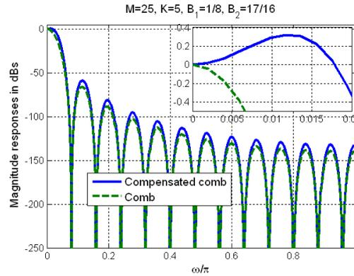
**Fig. 7** Magnitude responses of comb and compensator in [9]
