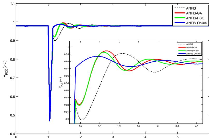
Fig. 6 Transient responses voltage at PCC ( $V_{PCC}$ )
