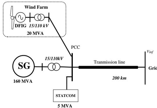
Fig. 5 Configuration of the OMIB system
