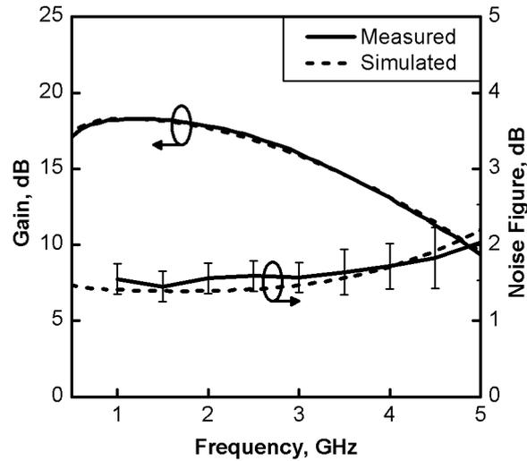
Fig. 3 Simulated and measured LNA gain and noise figure versus frequency
