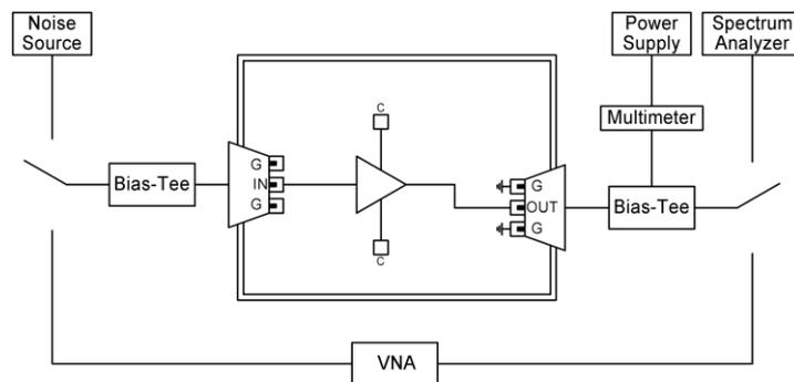
**Fig. 2** Experimental setup based on the microwave probe station
