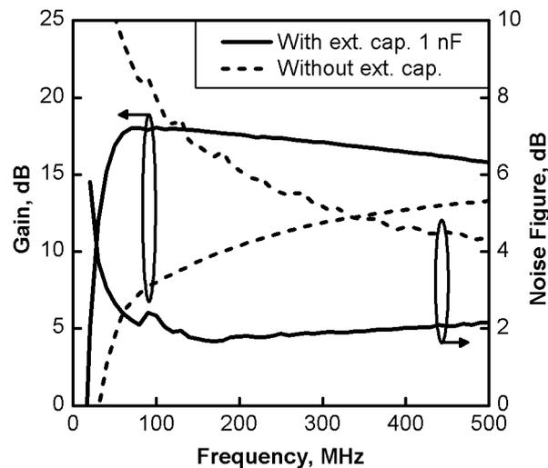
Fig. 7 Measured LNA gain and noise figure versus frequency
