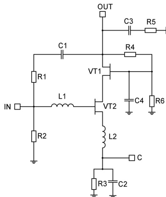
**Fig. 1** Simplified circuit of the LNA
