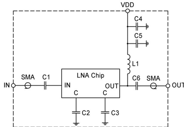
**Fig. 5** Special measurement test-fixtute schematic
