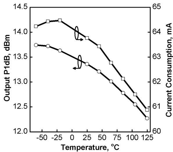
**Fig. 9** Measured LNA output  $P_{1dB}$  at 1 GHz and current consumption versus temperature
