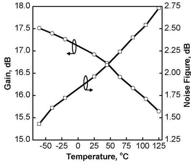
**Fig. 8** Measured LNA gain and noise figure at 1 GHz versus temperature
