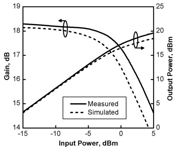
Fig. 4 Simulated and measured LNA gain and output power versus input power
