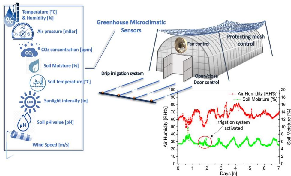
**Fig. 4** Block scheme of the smart autonomous agricultural system for improving yields in greenhouse based on sensor and IoT. Block scheme is based on [8]. The measured results for air humidity and soil moisture are given as an example.
