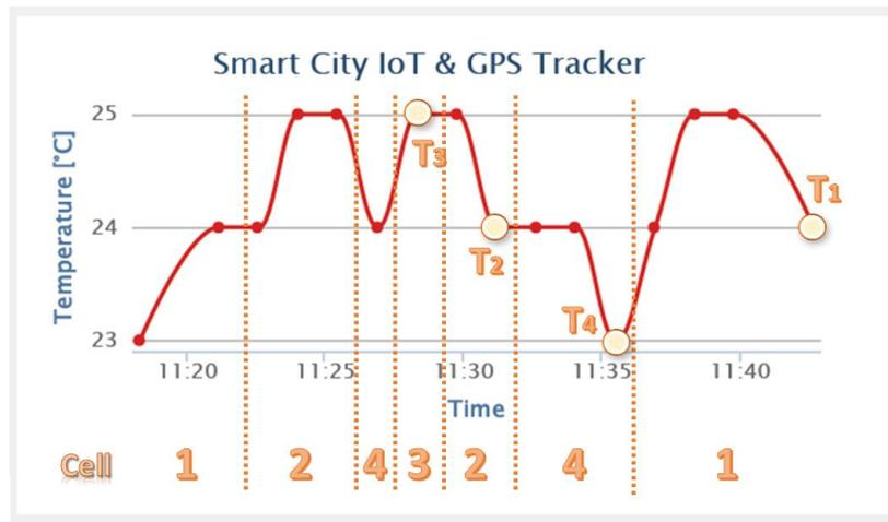
**Fig. 9** Measured temperature data with marked points that were last measured in specific cells
