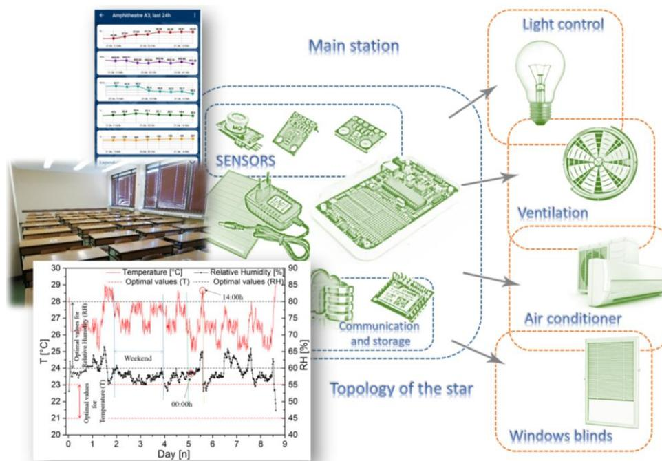
**Fig. 5** Block scheme of the smart data logger system based on sensor and Internet of Things technology as part of the smart faculty. Block scheme is based on [9]. The measured results for temperature and relative humidity are given as an example.
