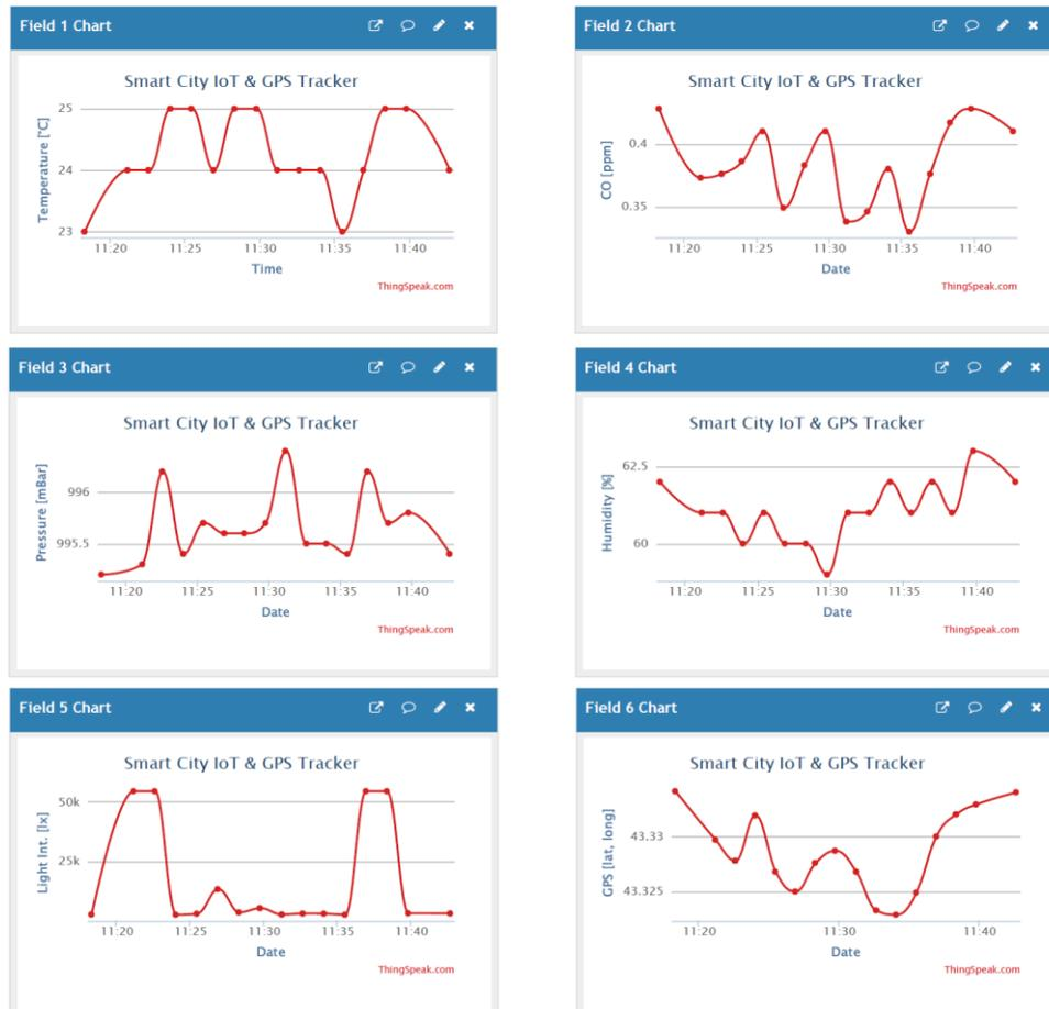
**Fig. 11** Measured parameters using the realized system (Temperature and CO concentration (Field 1 and Field 2) – first two charts, Air pressure and Air humidity (Field 3 and Field 4) – second two charts, Light intensity and GPS coordinates (Field 5 and Field 6) – third two charts)
