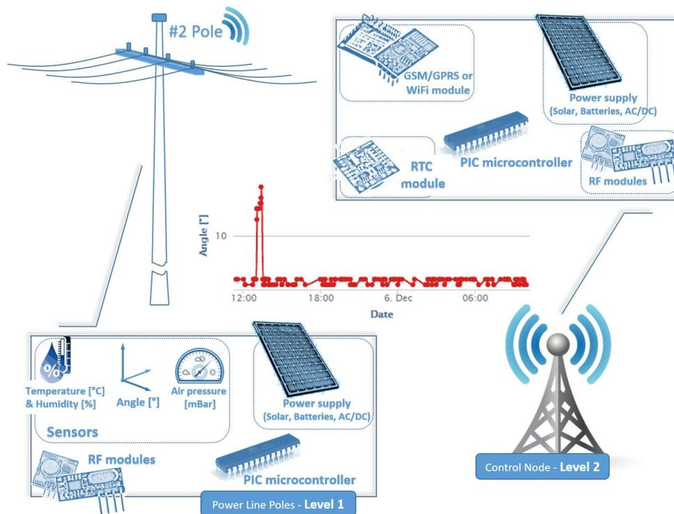
**Fig. 3** Block scheme of the smart system for supervision and monitoring of the power line poles using IIoT technology. Block scheme is based on [7]. The measured results for slope of angle are given as an example.
