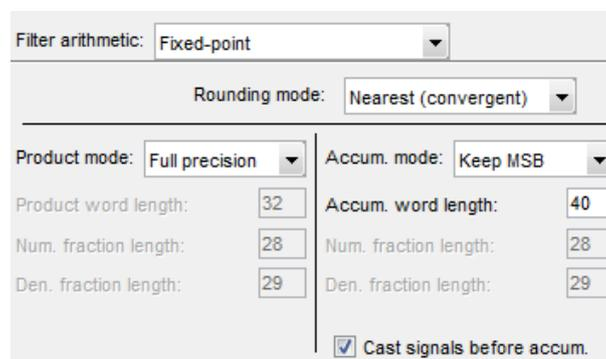
**Fig. 1** FDA Tool - setting simulation parameters of the multiplier
