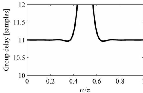
**Fig. 6** Group delay of the filter designed by zero positioning algorithm [9, 10]
