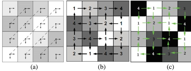
**Fig. 2** Regular Clocking Scheme (a) 2DDWave [20] (b) USE [18] (c) RES [19].
