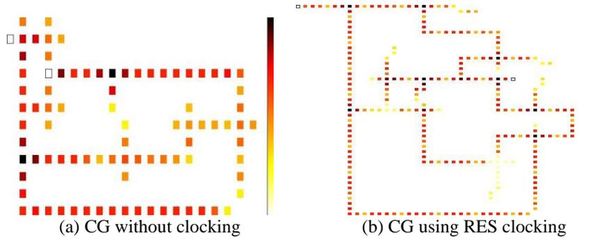
**Fig. 9** Energy Consumption map under tunneling energy  $0.5 E_k$ , at 2K temperature.
