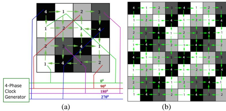
**Fig. 5** RES Clocking Scheme (a) Circuitry generates the electric fields for the clock (b) Extended version.
