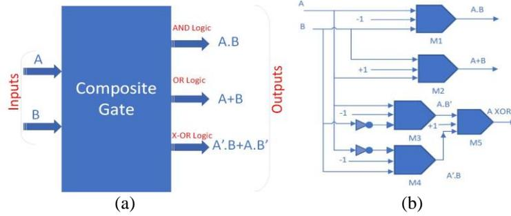
**Fig. 3** Composite Gate (a) Block Diagram (b) Schematic diagram.
