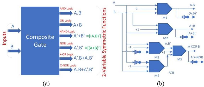
**Fig. 7** Composite Gate based realization of 2-variable symmetric functions (a) Block diagram (b) Schematic diagram.
