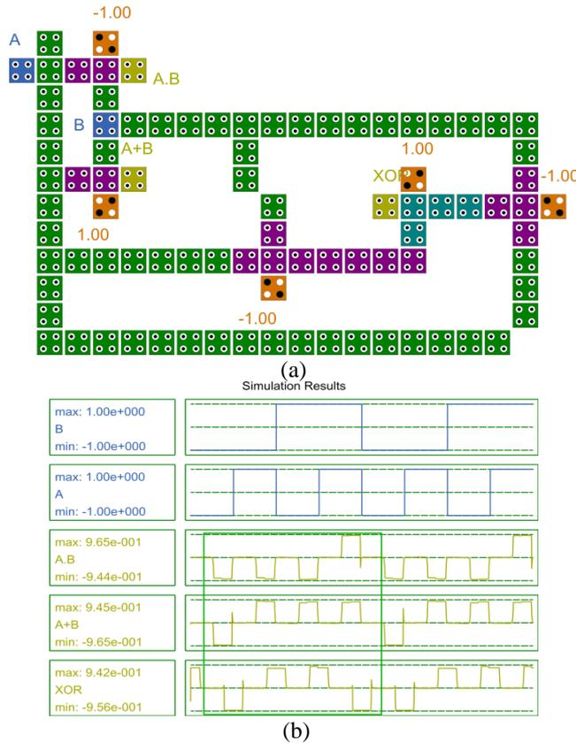
**Fig. 4** (a) QCA layout of the proposed Composite Gate (b) Simulated result.
