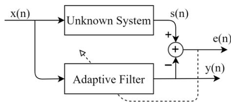
**Fig. 1** Adaptive system identification block diagram
