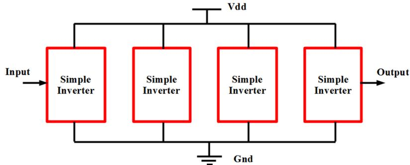
Fig. 13 General approach for a chain of 4 Inverters
