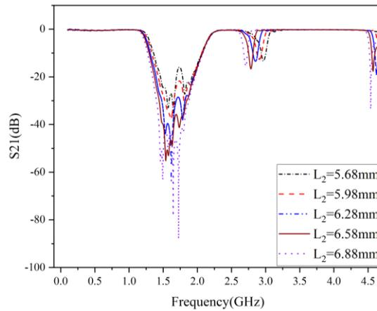
**Fig. 10** Variation of S21 parameters with length  $L_2$
