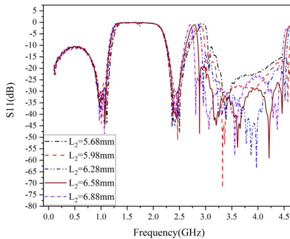
**Fig. 9** Variation of S11 parameters with length  $L_2$
