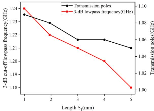
**Fig. 11** Simulation results for the  $S_1$  length optimization
