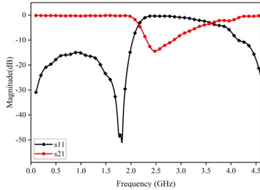
**Fig. 2** Simulated S-parameters of the lowpass filter
