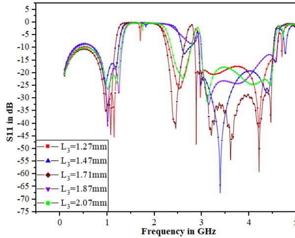
**Fig. 8** Variation of S11 parameters with length  $L_3$
