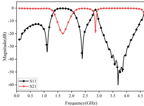
**Fig. 6** Simulated S-parameters of the proposed lowpass filter
