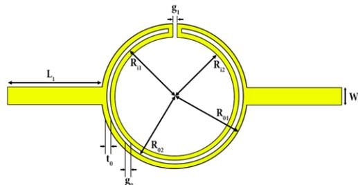
**Fig. 1** Schematic diagram of lowpass filter prototype with dimensions  $L_1=6.54$ ,  $t_0 = g_0 = g_1 = 0.3$ ,  $R_{01}= 5$ ,  $R_{02}= 4.7$ ,  $R_{11}= 4.4$ ,  $R_{12}= 4.1$ ,  $W_0=1.2$  (All dimensions are in mm).
