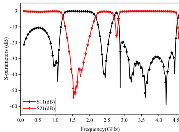
**Fig. 12** Frequency response of the proposed filter
