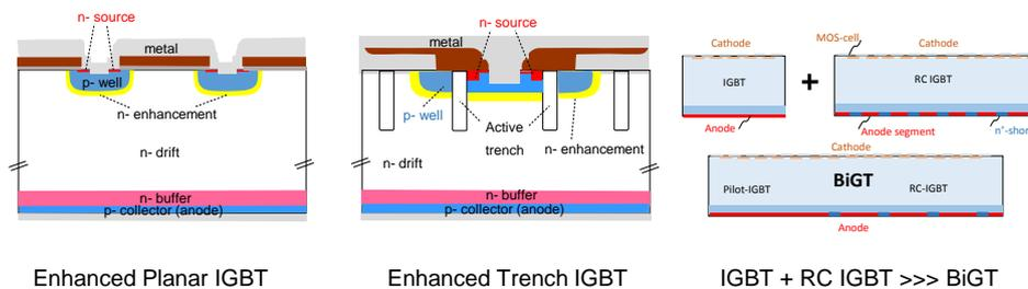
**Fig. 5** State-of-the-art IGBT design concepts
