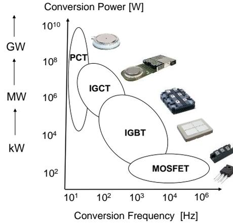
**Fig. 1** Power semiconductor devices
