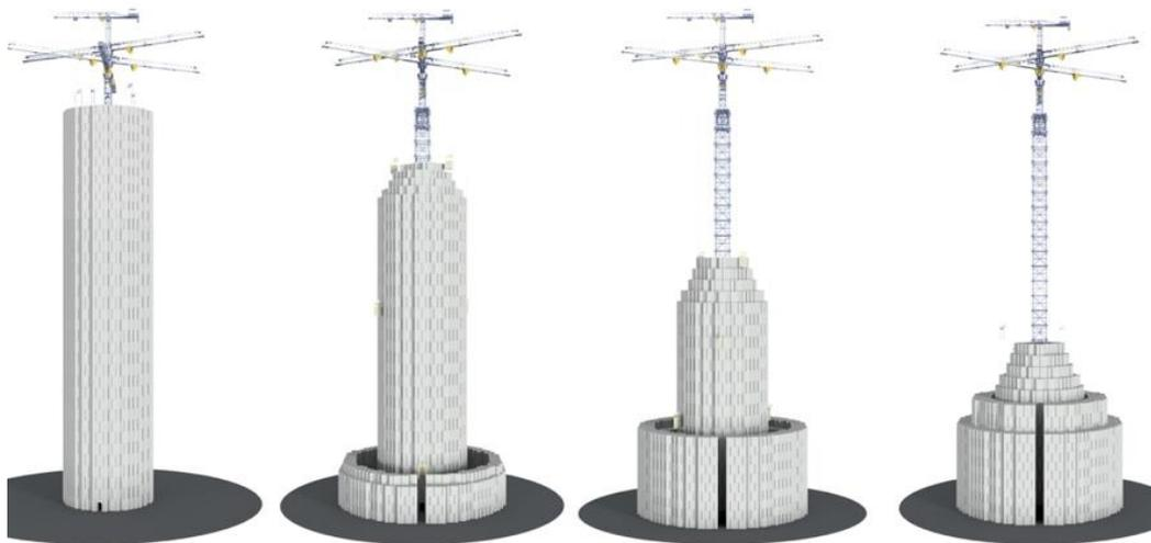
**Fig. 6** The Energy Vault system, a Dry Gravitational Storage System
