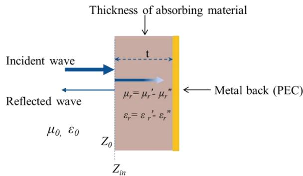
**Fig. 2** A schematic of single layer Dallenbach absorber
