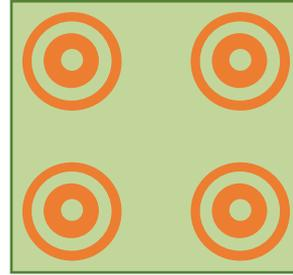
distinct resonant peaks. Dual and triple band metamaterial absorbers with wideband absorption was developed by Kollatou et al. by utilizing scalability property of metamaterials [45]. Special arrangements of donut-based resonators as shown in Figure 4 were also implemented in order to achieve multiband absorption. Multiple absorption peaks of 97%, 97%, 98% and 98% were observed at 6.5 GHz, 7.4 GHz, 9.2 GHz and 11.0 GHz respectively [46].
