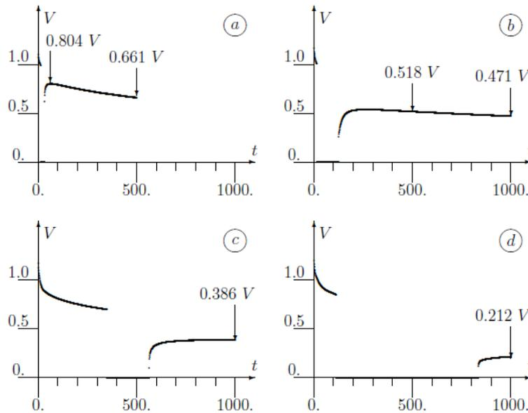
**Fig. 4** Transient voltages measured with short circuit periods of (a) 19 s, (b) 111 s, (c) 215 s and (d) 721 s
