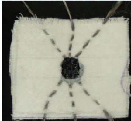
**Fig. 1** Photograph of a sample. Dimensions are about 5×5 cm<sup>2</sup>. The black area is the deposited PEDOT:PSS. Three stainless steel electrodes are sewed into the substrate.
