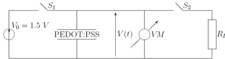
**Fig. 2** Schematic layout of the measuring circuit
