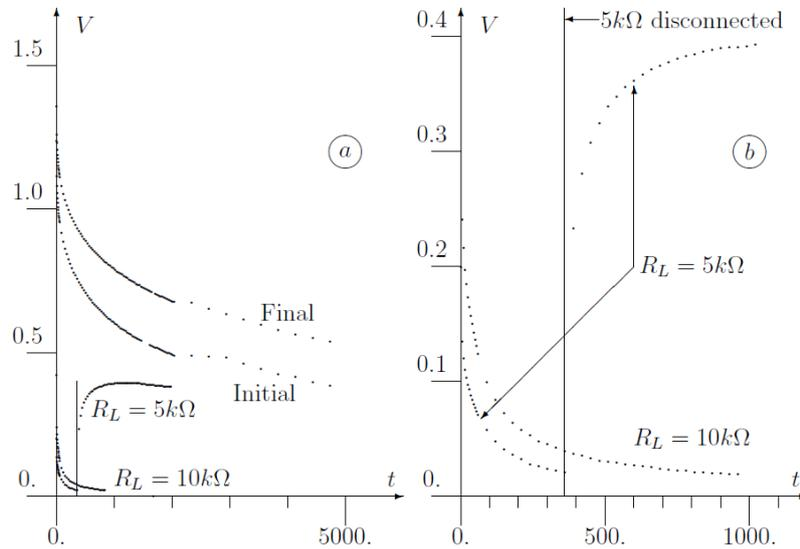
**Fig. 3** Voltage decay curves of PEDOT:PSS cells, with and without resistive load. (a) general view (b) detailed view of the dielectric absorption.
