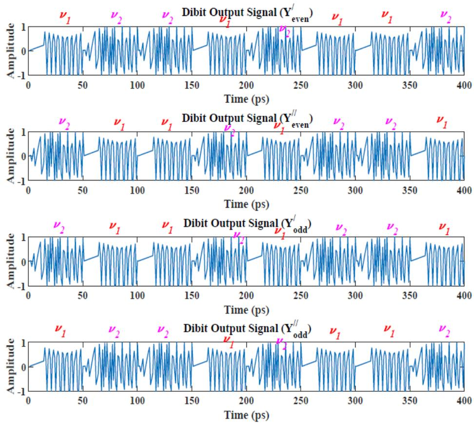
Fig. 5 Dibit output signal waveforms of parity generator
