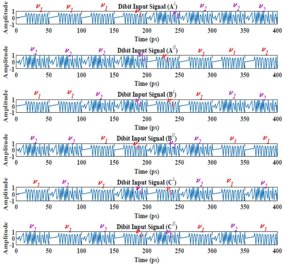
Fig. 4 Dibit input signal waveforms of parity generator
