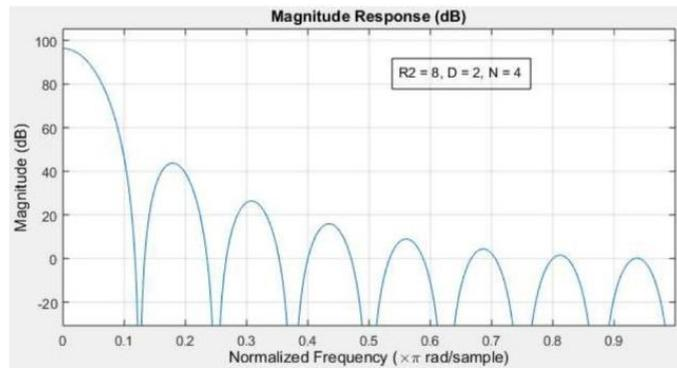
**Fig. 4** Magnitude response of the CIC filter for  $R_2 = 8, D = 2, N = 4$
