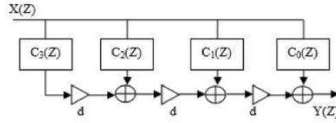
**Fig. 6** Cubic B-spline Farrow structure [20]
