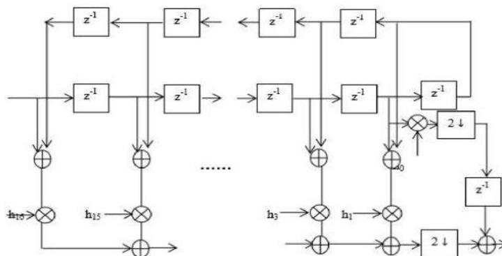
**Fig. 5** 31-tap transpose symmetric HB filter
