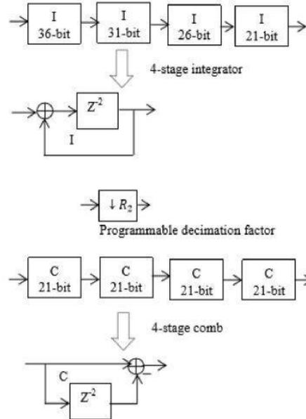
**Fig. 3** 4-stage truncated pipeline-based CIC filter
