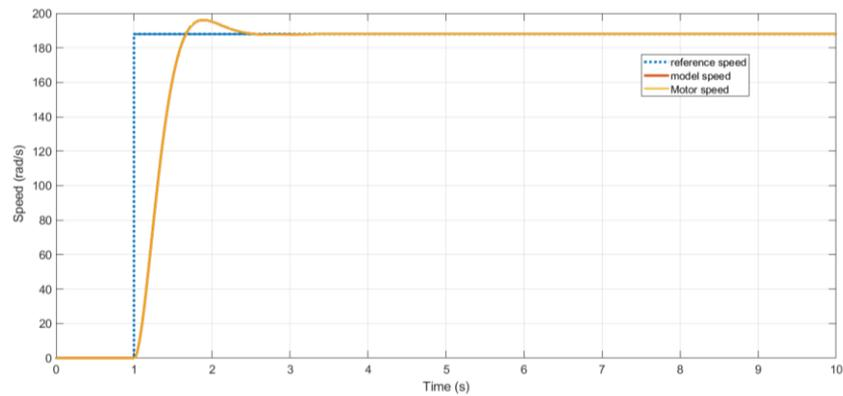
**Fig. 2** Speed response (Matlab Simulink)
