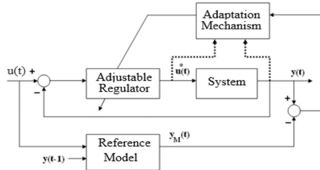
**Fig. 1** Principle of functioning of model reference adaptive control
