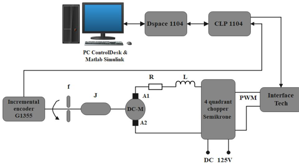
Fig. 4 Implementation adaptive control diagram on DCM
