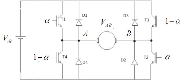
**Fig. 5** Four quadrant chopper drive DC motor
