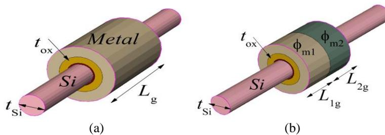
**Fig. 1** Schematic Structure of Cylindrical Gate All Around (GAA) MOSFET
