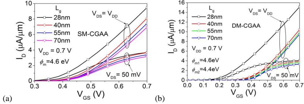
**Fig. 2** Drain current ( $I_D$ ) in linear scale as a function of gate to source voltage ( $V_{GS}$ ) for  $V_{DS}=50 \text{ mV}$  with variation in  $L_g$  (28 nm to 70 nm) (a) SM-CGAA ( $\phi_M=4.6 \text{ eV}$ ) (b) DM-CGAA ( $\phi_{M1}=4.6 \text{ eV}$ ,  $\phi_{M2}=4.4 \text{ eV}$ )
