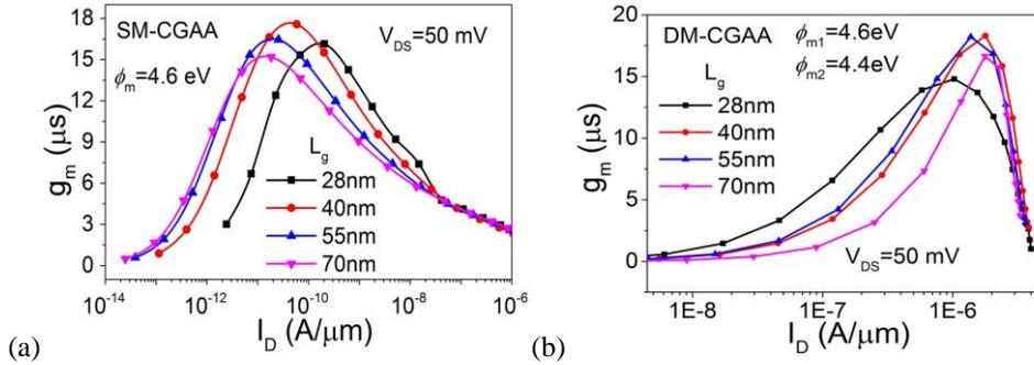
**Fig.5**  $g_m$  as a function of  $I_D$  at  $V_{DS}=50$  mV with variation in  $L_g$  (a) SM-CGAA ( $\phi_M=4.6$  eV) (b) DM-CGAA ( $\phi_{M1}=4.6$  eV,  $\phi_{M2}=4.4$  eV)
