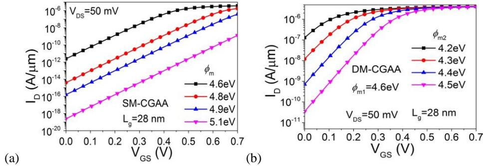
**Fig. 3** Drain current ( $I_D$ ) in log scale as a function of the gate to source voltage ( $V_{GS}$ ) for  $V_{DS}=50 \text{ mV}$  for different  $\phi_M$  (a) SM-CGAA (b) DM-CGAA
