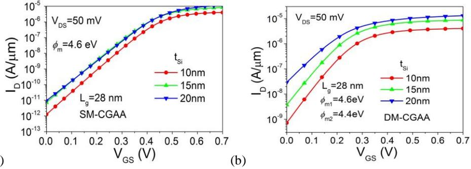
**Fig. 4** Drain current ( $I_D$ ) in log scale as a function of gate to source voltage ( $V_{GS}$ ) for  $V_{DS}=50$  mV with variation in  $t_{Si}$  (10 nm to 20 nm) (a) SM-CGAA ( $\phi_M=4.6$  eV) (b) DM-CGAA ( $\phi_{M1}=4.6$  eV,  $\phi_{M2}=4.4$  eV)
