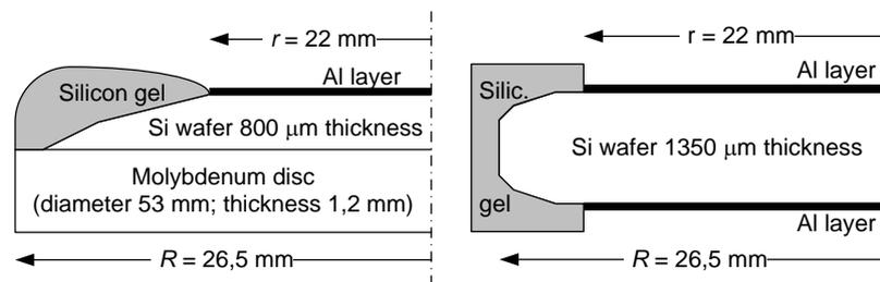
**Fig. 1** Cross-section of non-symmetrical structure of a 4kV PCR (left) and 6kV structure processed by strictly symmetrical free-floating technology (right).
