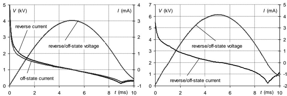
**Fig. 3** Pulse measurement at the analyzer Schuster SML 698: Reverse and off-state voltage and current waveforms (4kV PCR left; 6kV PCR right).
