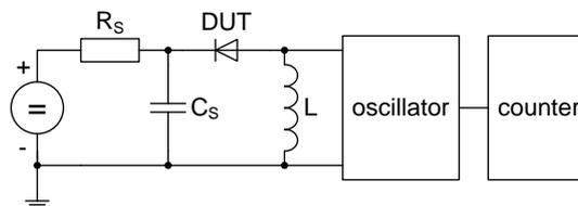
**Fig. 6** Resonance method of measurement capacity of a biased p-n junction.
