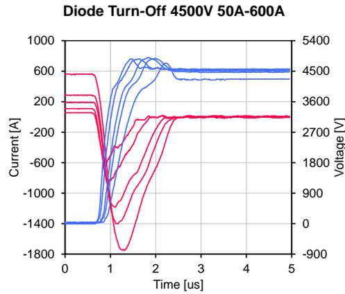
**Fig. 8** 6.5kV/600A BIGT module diode-mode turn-off waveforms at critical low current conditions at  $-40^{\circ}\text{C}$ .
