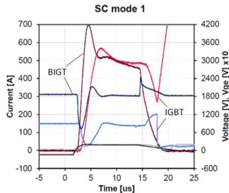
**Fig. 9** 3.3kV IGBT and BIGT single chip Short Circuit type 1 waveforms at room temperature.
