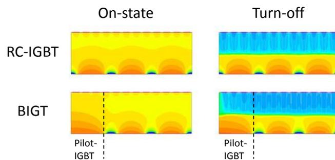
**Fig. 5** Hole density during IGBT on-state conduction and turn-off of a Reverse-Conducting IGBT compared to the BIGT, showing the effect of carrier plasma un-uniformity and the occurrence of dynamic avalanche.
