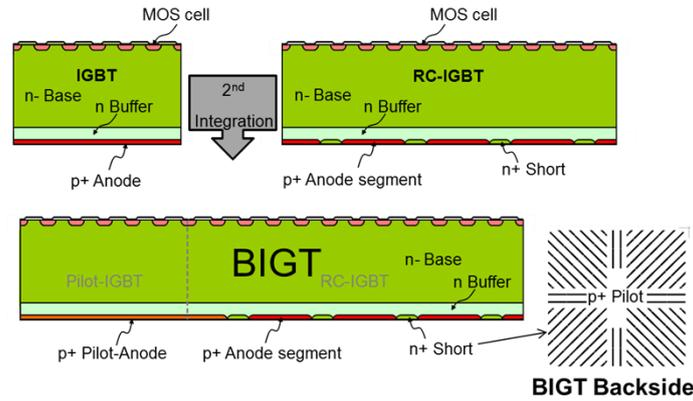
Fig. 3. Second integration step: the bimode insulated gate transistor BIGT.
