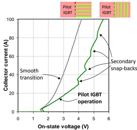
Fig. 4 Reducing the snap-back with the BIGT hybrid design and radial shorting layout.
