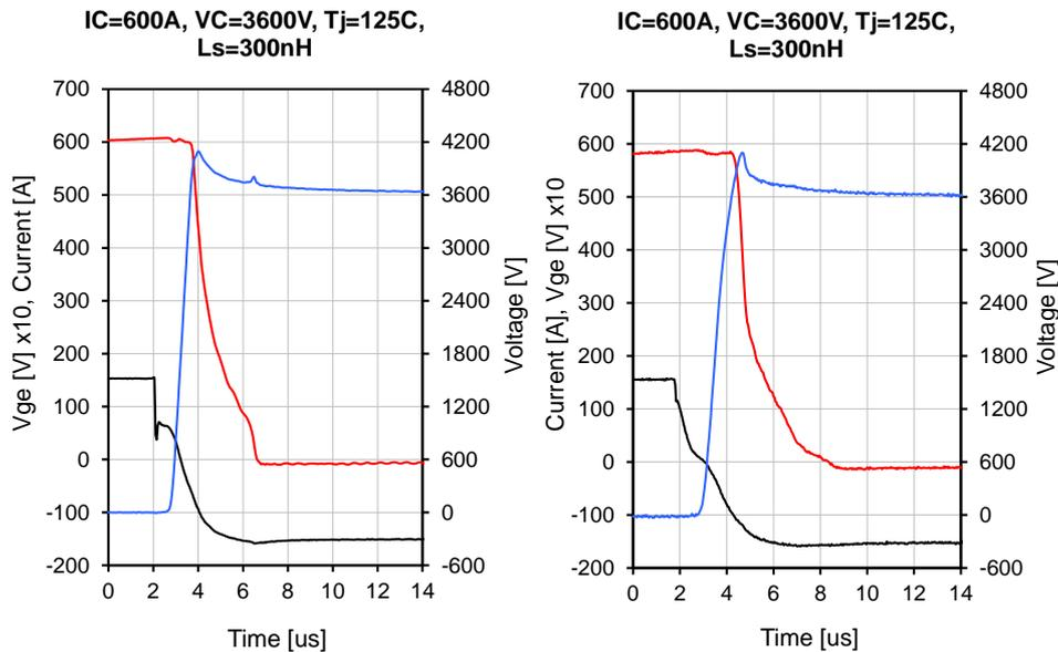
**Fig. 7** 6.5kV/600A IGBT (left) and BIGT (right) module turn-off waveforms under nominal conditions.
