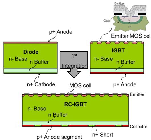
**Fig. 2** First integration step: the reverse conducting RC IGBT.
