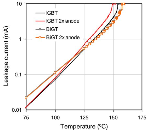
Fig. 6 6.5kV BIGT and IGBT thermal stability curves.
