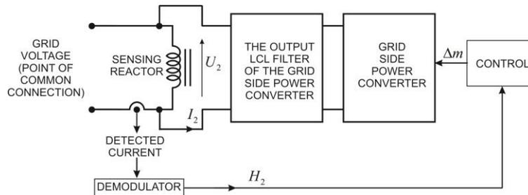
**Fig. 7** Using the grid connected power converter as an actuator in closed loop DC bias suppression system. Control circuit detects the second harmonic, concludes on the DC bias, and produces the DC voltage correction  $U_2$ . This voltage injects the DC current  $I_2$  which zeroes out the DC bias detected across the grid connection.
