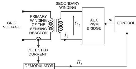
**Fig. 6** Using the sensing reactor with the compensating winding. Control circuit sets the voltage  $U_2$  in order to obtain the current  $I_2$  of the compensating winding which zeroes out the offset from the sensing core.
