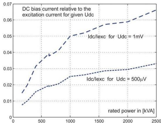
**Fig. 2** The ratio between the DC bias current and the rated magnetizing current for DC offset voltages of 500  $\mu$ V and 1 mV.
