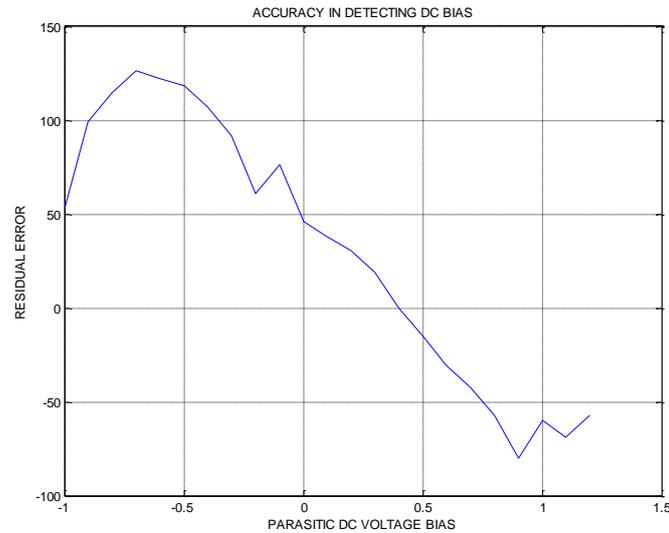
**Fig. 9** Residual error obtained in the steady state, with the circuit given in Fig. 6. On x-axis, parasitic DC bias in 0.4kV AC grid is given, expressed in [mV]. Residual error is given on y-axis in [ $\mu\text{V}$ ].
