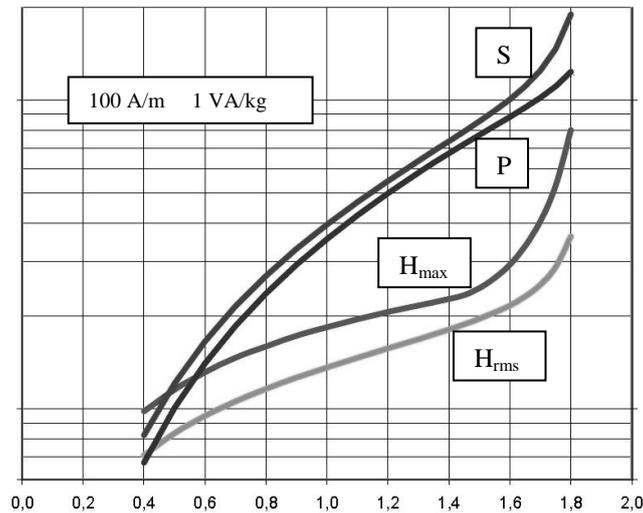
**Fig. 3** Peak value of the magnetic field, rms value of the magnetic field, specific power losses and specific apparent power  $S$  as a function of the flux density.
