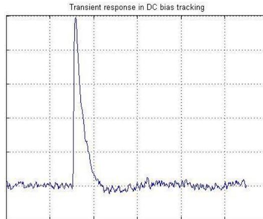
**Fig. 8** Transient response of the DC bias suppression controller. The scaling of x-axis is 500ms per division. The vertical axis shows detected DC bias with the scaling of 0.5mV per division. An artificial bias of 2.5mV is introduced into the systems, and it is removed in, roughly, 200ms.
