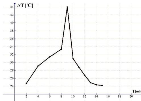
**Fig. 3** Temperature increments  $\Delta T$  for power supply for which the fail of thermistor was triggered off after 8 minutes of power supply operating.
