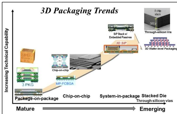
**Fig. 3-1** 2.5/3D packaging technologies showing conventional to advanced configurations.
