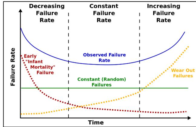
**Fig. 6.2** Classic bathtub reliability curve showing the three stages during the life of a product from a reliability perspective: infant mortality, steady-state, and wear-out.
