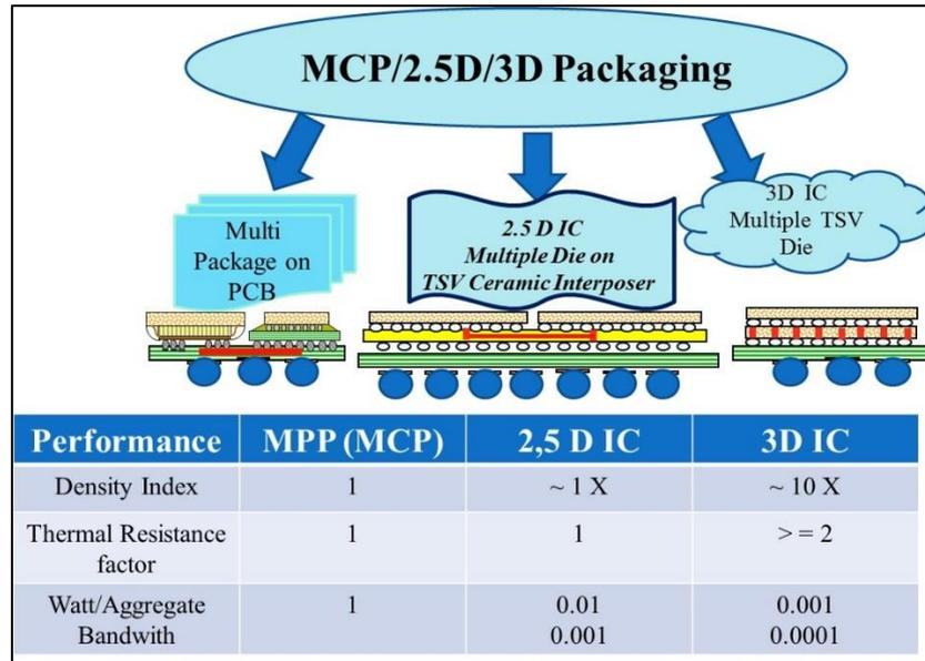
**Fig. 3-4** 2.5/3D packaging technologies showing conventional to advanced configurations.
