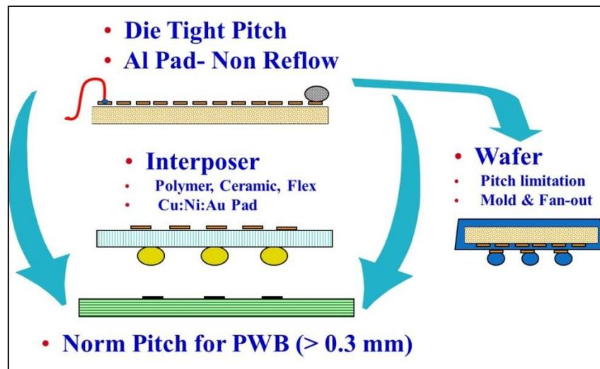
**Fig. 2-1** Single-chip packaging concept from wire-bond to flip-chip ball grid array to wafer-level packaging (fan-in and fan-out).
