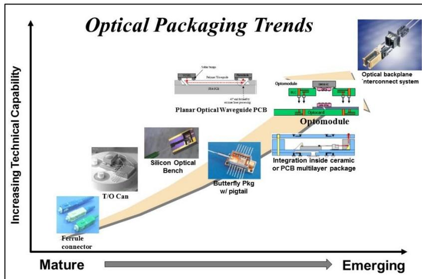
**Fig. 5-2** Optical packaging trends from conventional to advanced packaging technologies.
