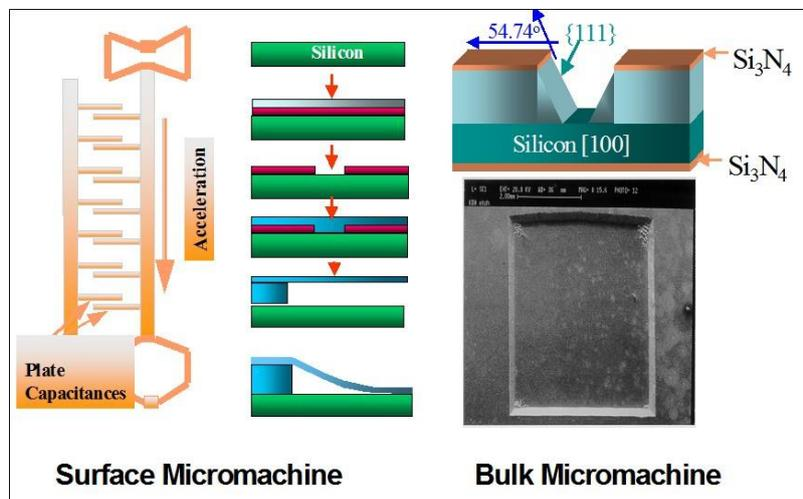
**Fig. 5-1** Surface and bulk micromachining fabrication and structure
