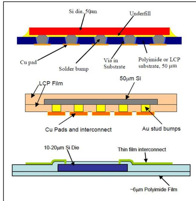
**Fig. 4-3** Three techniques of thinning die: polyimide and LCP substrate with solder assembly (top); LCP substrate with thermal compression bond Au stud bump assembly (middle); thinned Si die embedded in polyimide with thin film interconnect (bottom) [38].
