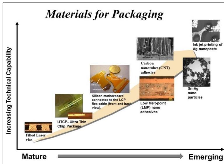
Fig. 5-5 Materials for packaging technologies
