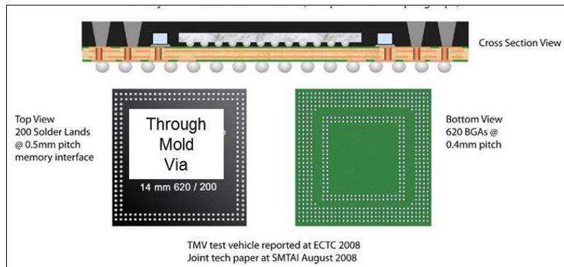
**Fig 3-3** Cross-section top and bottom view of a new TMV™ PoP package [19].
