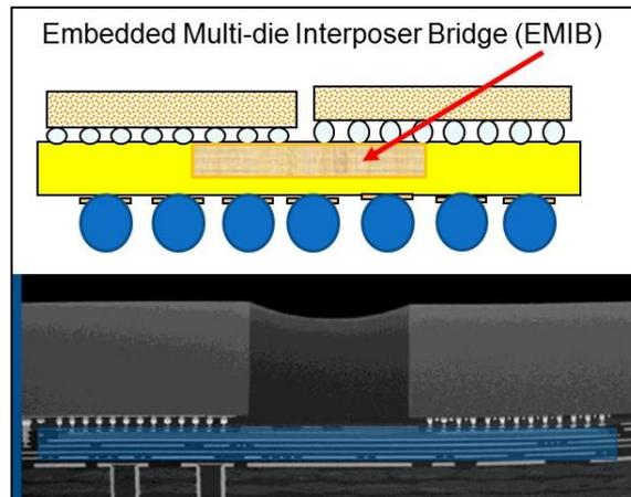
**Fig. 3-6** A low-cost 2.5D laminate with silicon embedded bridge for effective flip-chip routing [27]
