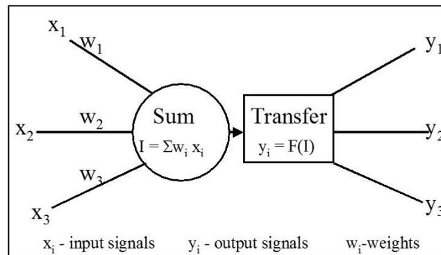
**Fig. 7-1** Schematic of an ANN structure
