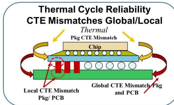
**Fig. 6-1** Three key elements define reliability under thermal stress are due to global, local, and solder alloy coefficient of thermal (CTE) mismatches.
