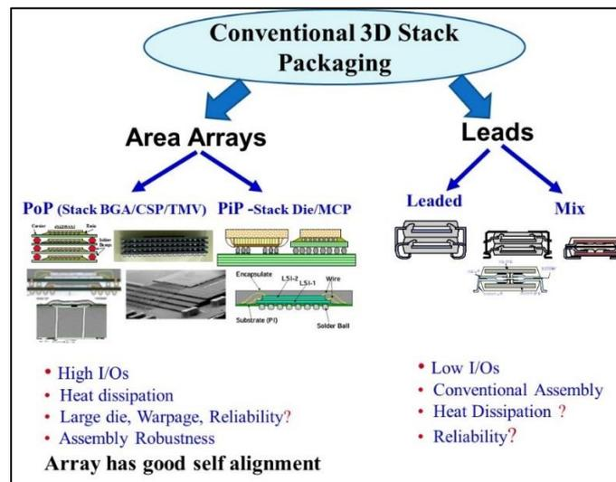
**Fig. 3-2** 2.5/3D packaging technologies showing conventional to advanced configurations.
