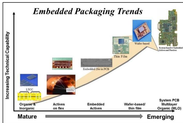
Fig. 4-2 Embedded passive and active in printed circuit board and package.
