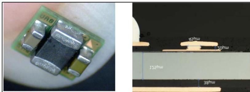
**Fig. 4-5** Configuration of wafer level chip scale module package (WLCSMP).
