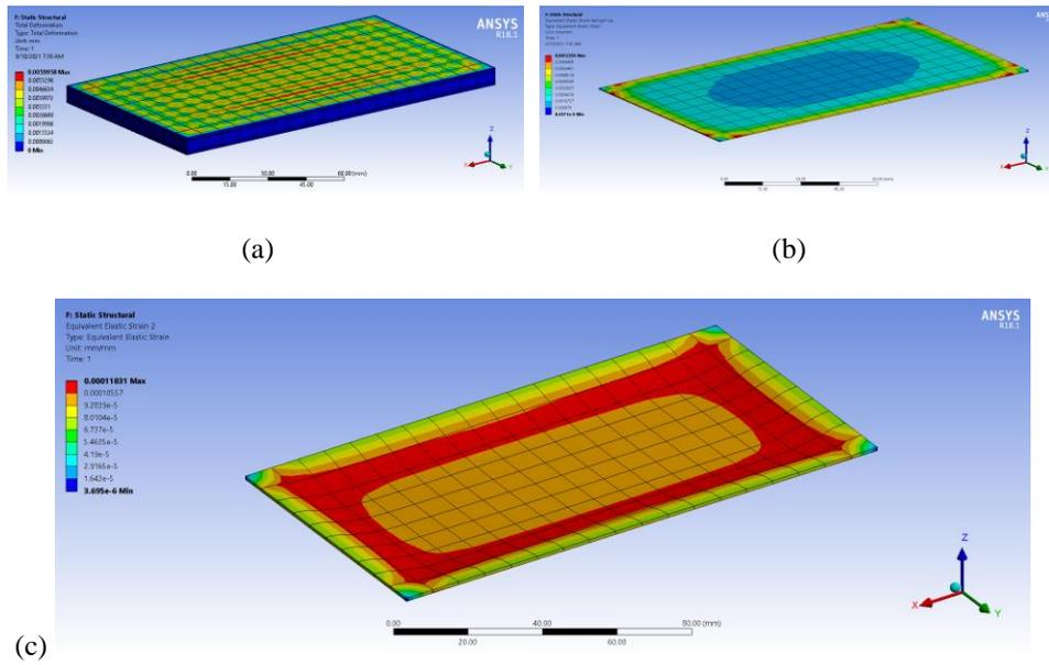
**Fig. 18** Sandwich with aerogel layer. (a) Sandwich structure showing deformation on the top face at 427 °C (carbon foam core and aerogel layer used); (b) Thermal strain on top aerogel layer; (c) thermal strain on bottom skin
