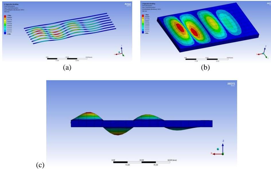
**Fig. 6** (a) Cylindrical carbon fiber imbedded in the core (diameter of 1.5 mm); (b) Buckling of sandwich under axial compression (isometric view); (c) Buckling of sandwich under axial compression (side view)
