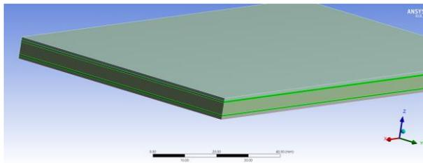
Fig. 16 Sandwich structure with silica aerogel layer
