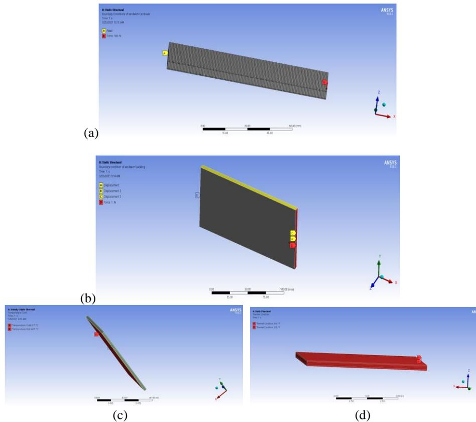
**Fig. 2** Boundary conditions (a) cantilever for bending analysis; (b) simply supported, moving along horizontal direction; (c) steady-state temperature boundary condition (higher temperature applied on top skin); (d) Thermal expansion of sandwich beam
