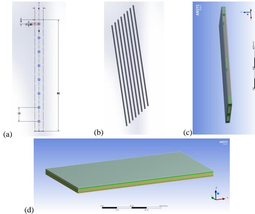
**Fig. 1** Geometry of sandwich beam (a) Cylindrical bar strut of 1.5 mm diameter and 10 mm spacing; (b) Carbon fiber strut imbedded in core; (c) Rectangle shape strut inserted in core (d) Sandwich with added aerogel layers
