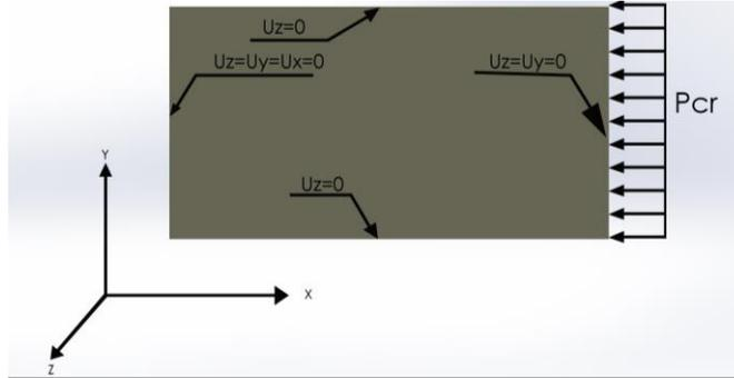
**Fig. 3** Schematic model of buckling setup
