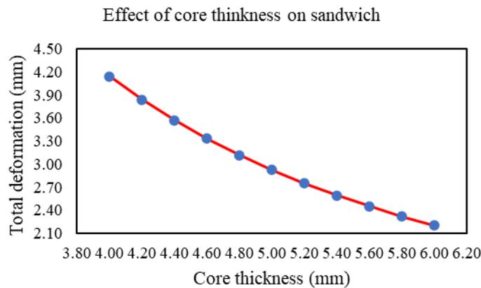
**Fig. 12** Core thickness (mm) vs. total deformation (mm)
