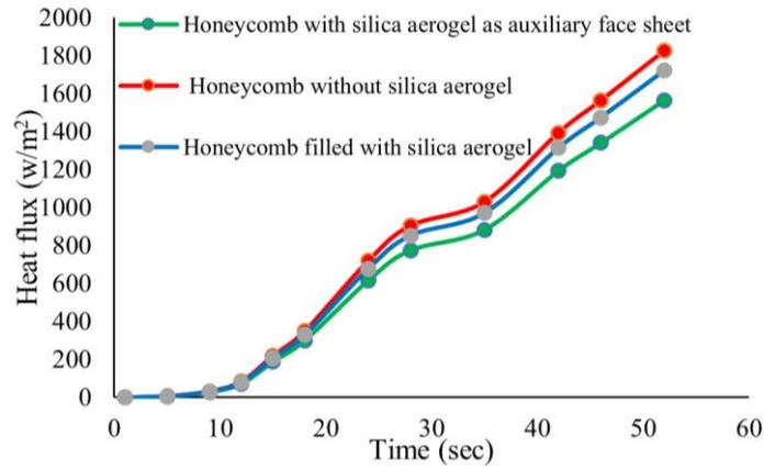
Fig. 21 Time vs. heat flux of sandwich panel
