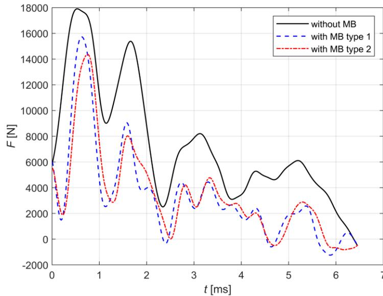
**Fig. 6** Experimental averaged recoil forces
