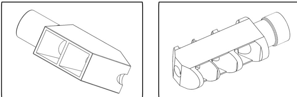
**Fig. 1** Muzzle brake types: (left) Type 1, (right) Type 2
