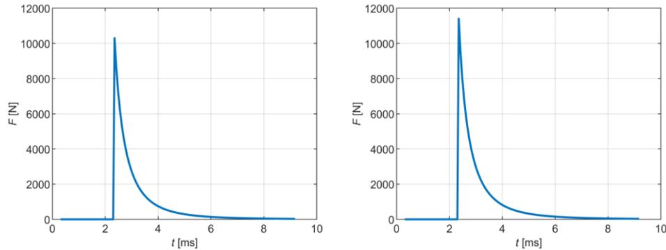
**Fig. 2** Muzzle brake forces: (left) MB type 1, (right) MB type 2
