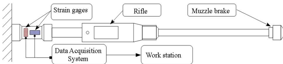
**Fig. 3** Schematic of experiment setup
