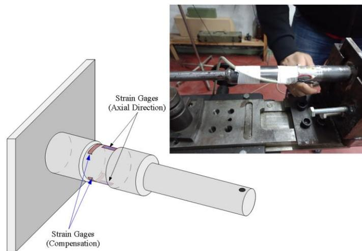
**Fig. 5** Force measurement sensor: (left) schematic, (right) picture
