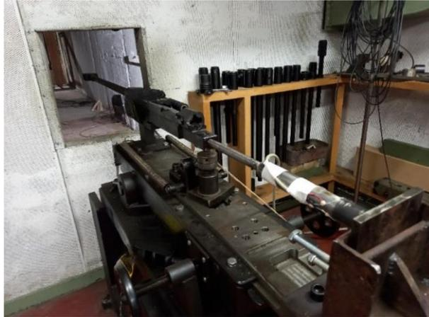
**Fig. 4** Recoil measurement apparatus
