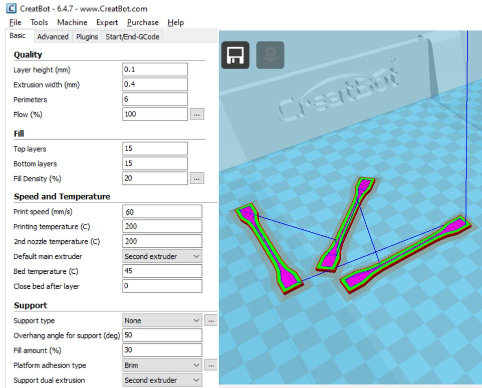
**Fig. 2** Generation of the G-code in the *CreatWare* software of the *CreatBot DX2 3D* printer
