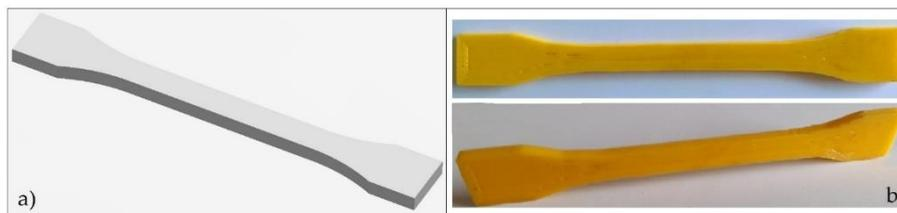
**Fig. 1** Test specimen: a) *STL* model; b) a sample made on a 3D printer
