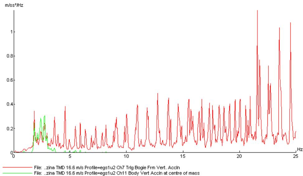
**Fig. 13** Compiled frequency spectrum of bogie frame and center of the mass of vertical acceleration
