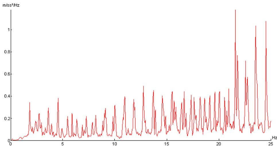
**Fig. 5** Vertical acceleration in frequency domain at speed of 60 km/h
