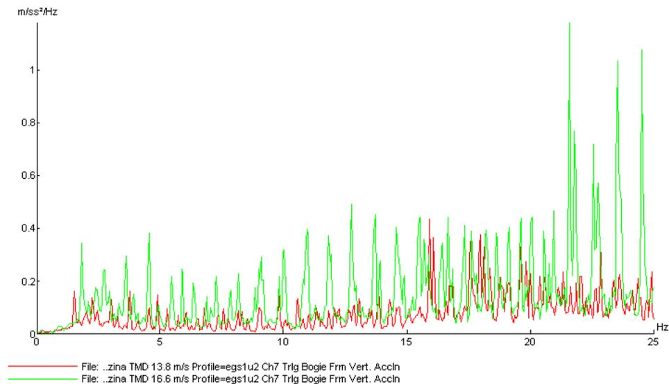
**Fig. 11** Frequency spectrum of vertical acceleration of bogie frame
