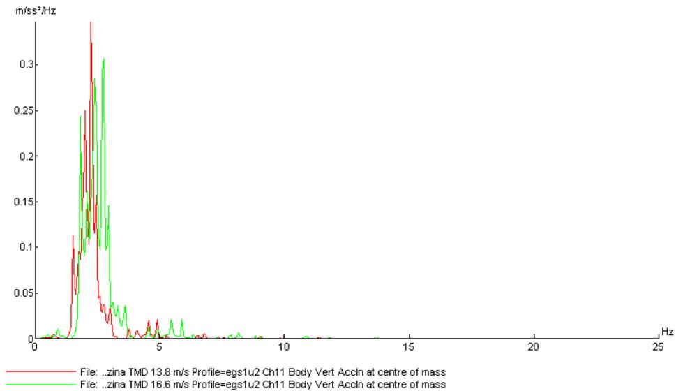
**Fig. 12** Frequency spectrum of vertical acceleration at center of mass
