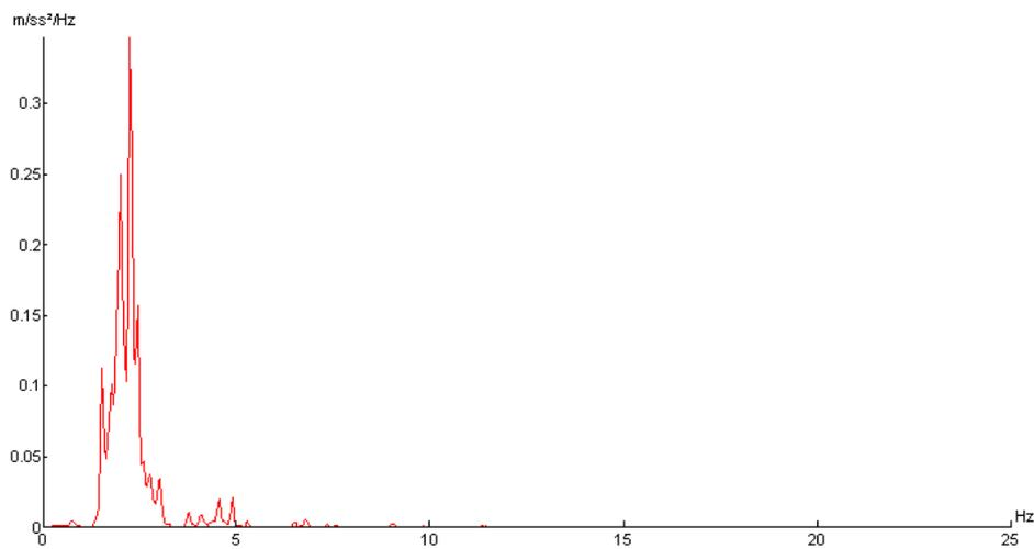
**Fig. 8** Vertical acceleration in the frequency domain (50 km/h)
