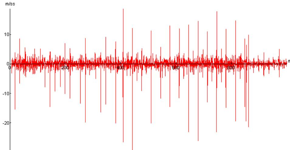
**Fig. 2** Vertical acceleration with respect to distance traveled 0-1000m
