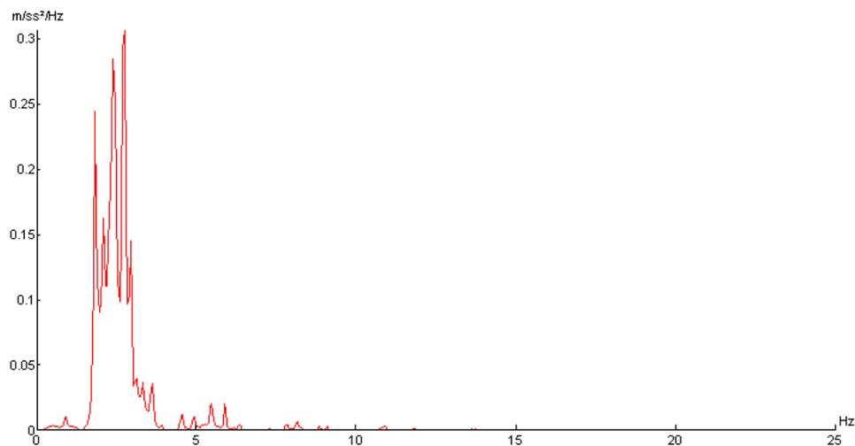
**Fig. 10** Vertical acceleration in frequency domain (60 km/h)
