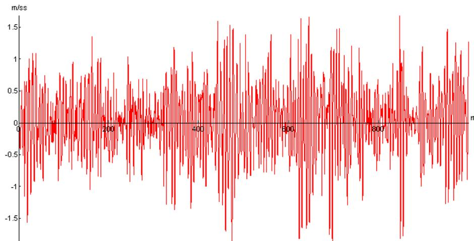
**Fig. 7** Vertical acceleration with respect to distance traveled 0-1000 m
