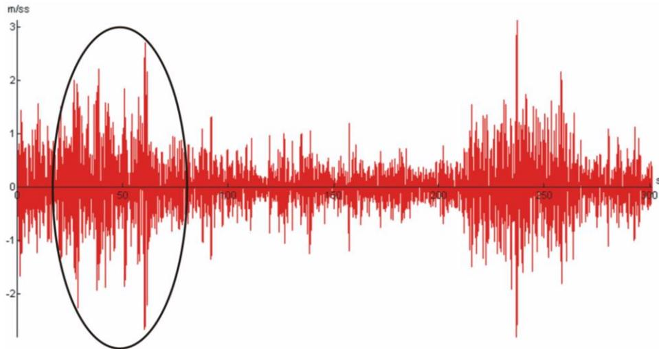
**Fig. 9** Vertical acceleration in time domain (60 km/h)
