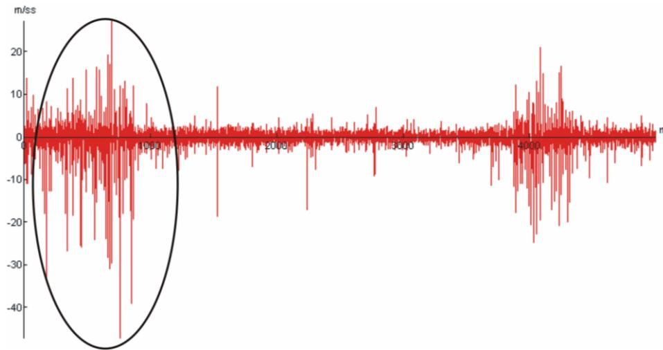
**Fig. 4** Vertical accelerations at speed of 60 km/h
