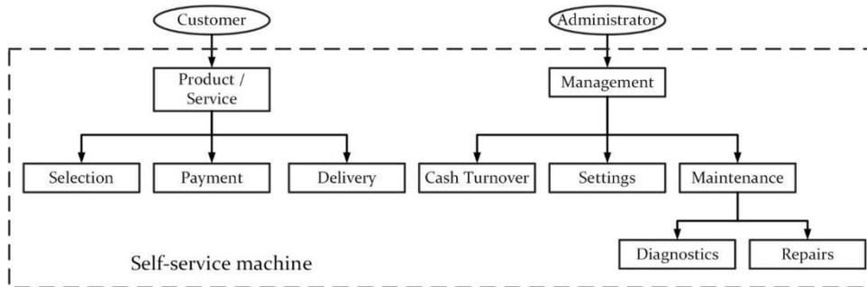
**Fig. 6** Two types of users on the self-service automated system/vending machines
