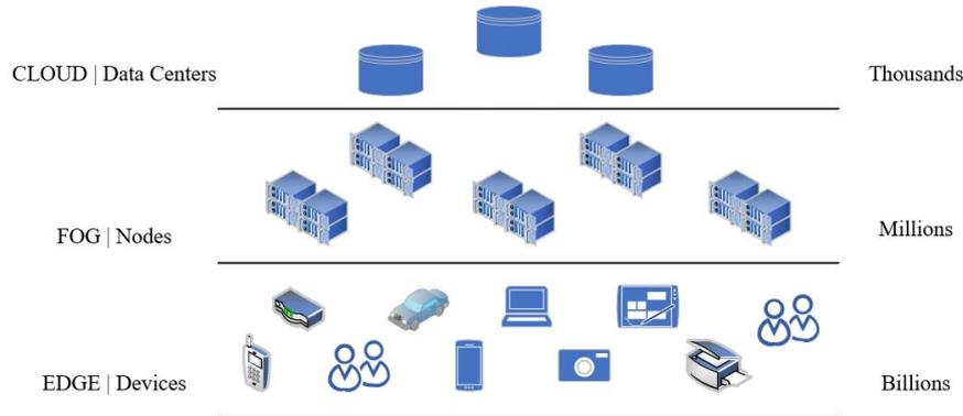
**Fig. 1** IoT-Edge-Fog-Cloud architecture based on [12]
