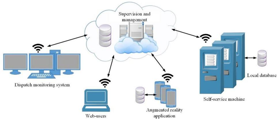
**Fig. 10** Architecture of the smart-shop network system
