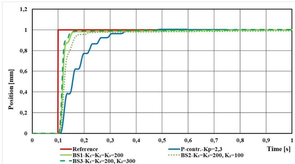
Fig. 5 Step response of EHS system by different values of  $K_2$
