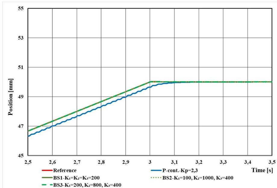
Fig. 9 Detail by approaching the final value of a ramp response of the EHS system with different values of  $K_2$  and  $K_3$
