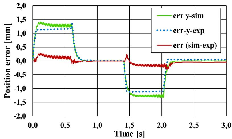
Fig. 3 The error of simulated and experimental response to reference
