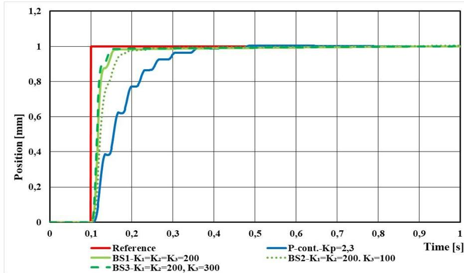
**Fig. 6** Step response of EHS system by different values of  $K_3$
