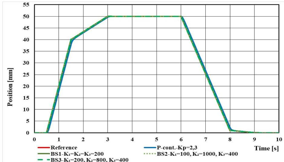
Fig. 8 Ramp response of EHS system with different values of  $K_2$  and  $K_3$
