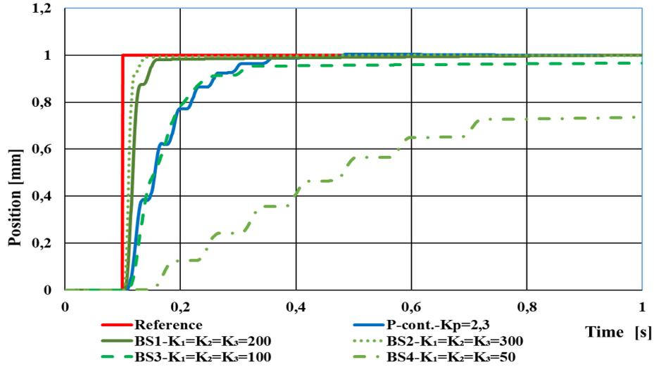
Fig. 4 Step response of EHS system by the backstepping controller
