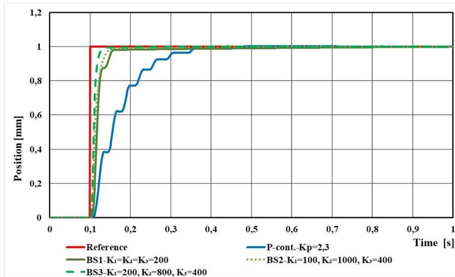
**Fig. 7** Step response of EHS system with different values of  $K_2$  and  $K_3$
