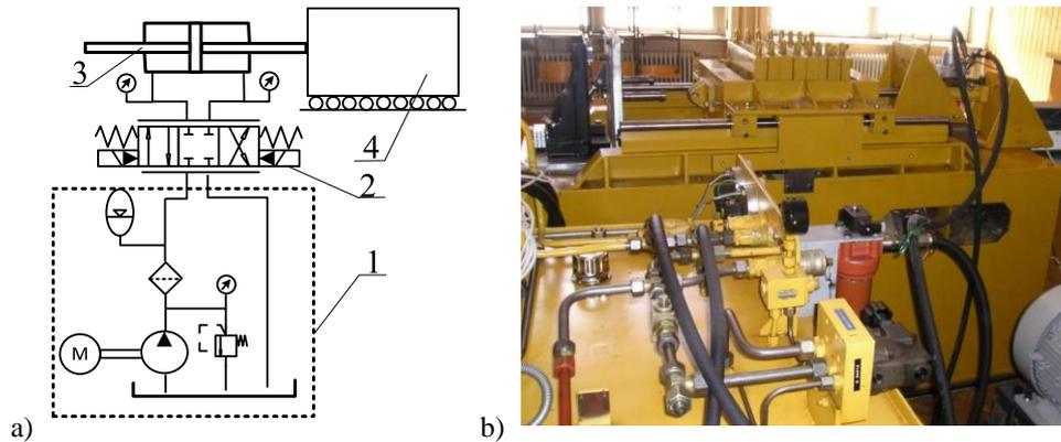
**Fig. 1** a) EHS positioning system b) Electrohydraulic servo system with load
