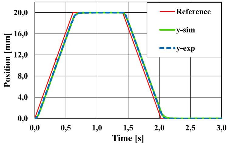
Fig. 2 Comparison of nonlinear mathematical model and the experimental response of the EHS system with ramp response
