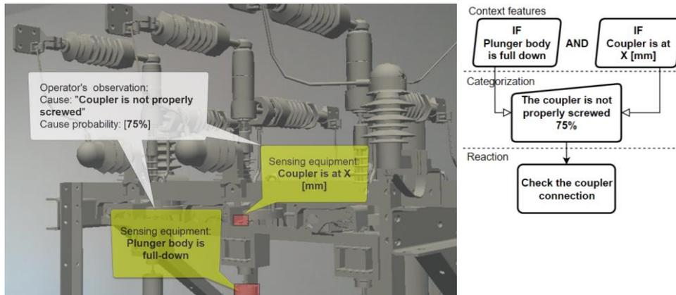
**Fig. 9** Operator's observation based on captured data from the sensing equipment can be formalized into an expert rule for reaction (MR-app for the case of assembling three phase recloser. MS HoloLens was used as MR-app running hardware.)
