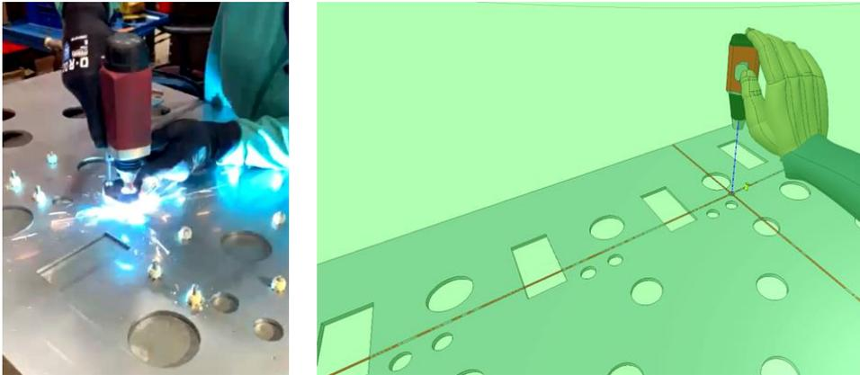
**Fig. 5** Guiding the welder towards proper dents in the sheet metal plate. (MR-app hand-welding of studs onto tank sheet plates. MS HoloLens was used as MR-app running hardware.)
