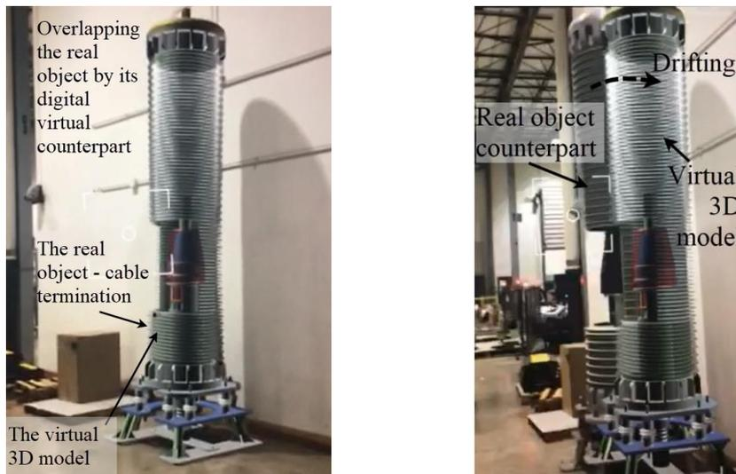
**Fig. 4** Coinciding the 3D digital model of high-voltage cable termination with its real counterpart. (AR-app for remote assistance in handling the issues with high voltage cable termination. iPad Pro™ was used as AR-app running hardware.)
