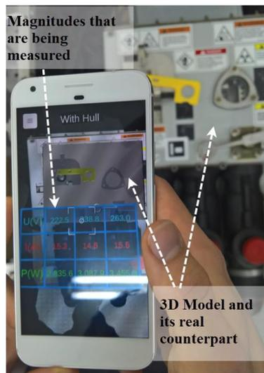
**Fig. 3** The virtualized high-voltage switchgear with the magnitudes that are being measured by its sensors. (AR-app for diagnosing the high-voltage equipment status in the field. iPhone and Android phones were used as AR-app running hardware.)
