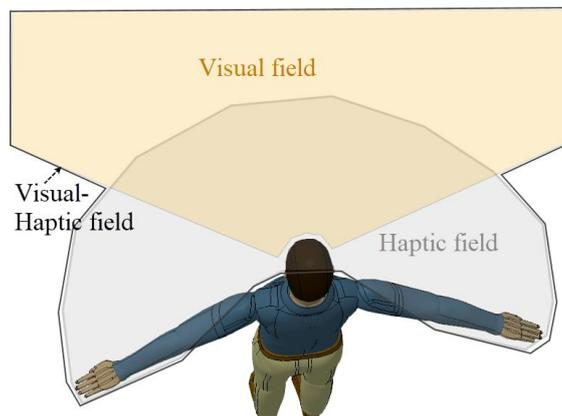
**Fig. 1** The space of visual and haptic field of an operator – VHF
