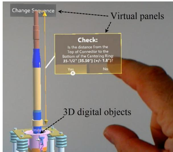
**Fig. 2** Digital content (alpha-numerical and graphical data and 3D objects) in VHF. (MR-app for assembling the high-voltage equipment. MS HoloLens was used as MR-app running hardware.)
