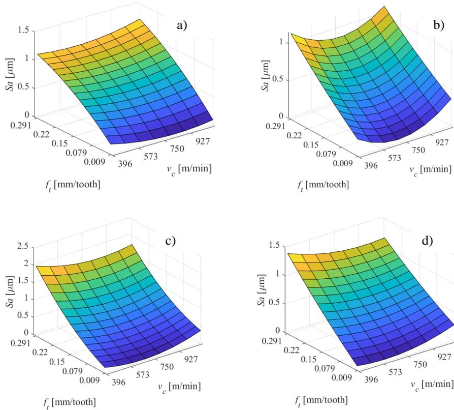
**Fig. 5** Influence of feed per tooth and cutting speed on surface roughness  $S_a$  using dry machining a) and cooling techniques: b) CCA, c) CF, d) MQL
