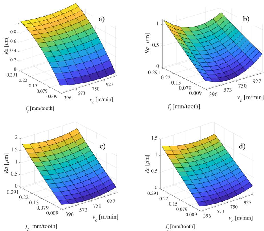
**Fig. 4** Influence of feed per tooth and cutting speed on surface roughness  $Ra$  using dry machining a) and cooling techniques: b) CCA, c) CF, d) MQL
