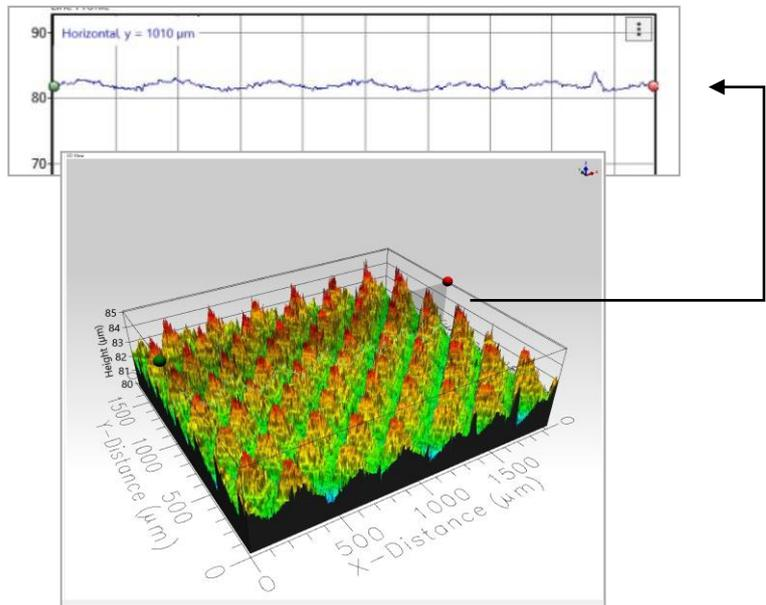
**Fig. 11** Surface scan of dry down milled specimen at 750 m/min and 0.15 mm/tooth. Surface roughness measured for this test were  $Ra = 0.647 \mu\text{m}$  and  $Sa = 0.754 \mu\text{m}$
