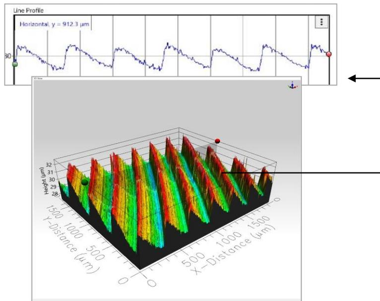
**Fig. 10** Surface scan of dry down milled specimen at 396 m/min and 0.15 mm/tooth. Surface roughness measured for this test were  $Ra = 0.896 \mu\text{m}$  and  $Sa = 0.808 \mu\text{m}$
