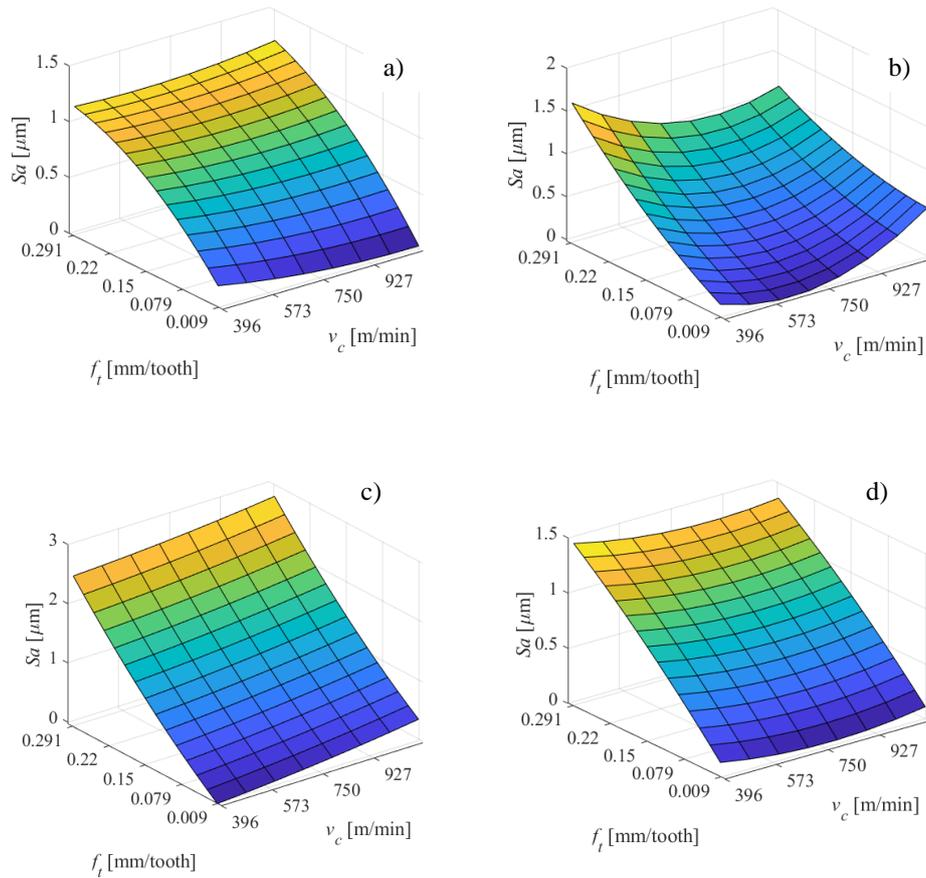
**Fig. 3** Influence of feed per tooth and cutting speed on surface roughness  $Sa$  using dry machining a) and cooling techniques: b) CCA, c) CF, d) MQL
