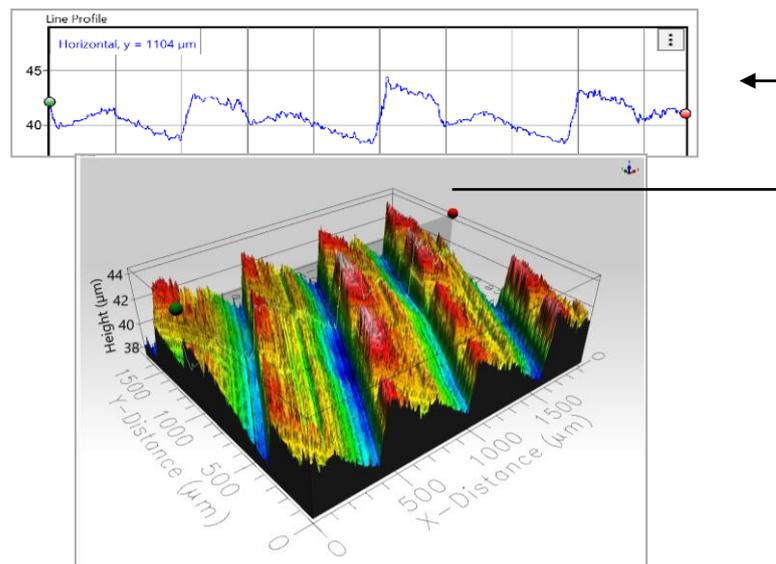
**Fig. 9** Surface scan of dry down milled specimen at 750 m/min and 0.29 mm/tooth. Surface roughness measured for this test were  $Ra = 1.310 \mu\text{m}$  and  $Sa = 1.052 \mu\text{m}$
