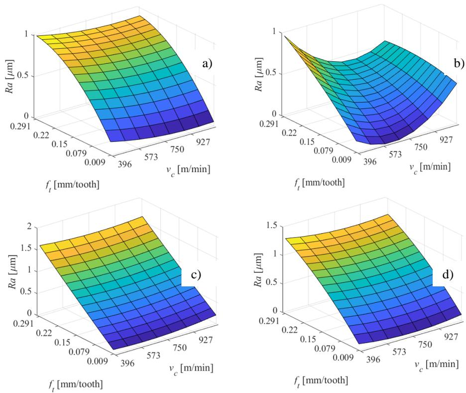
**Fig. 2** Influence of feed per tooth and cutting speed on surface roughness  $Ra$  using dry machining a) and cooling techniques: b) CCA, c) CF, d) MQL
