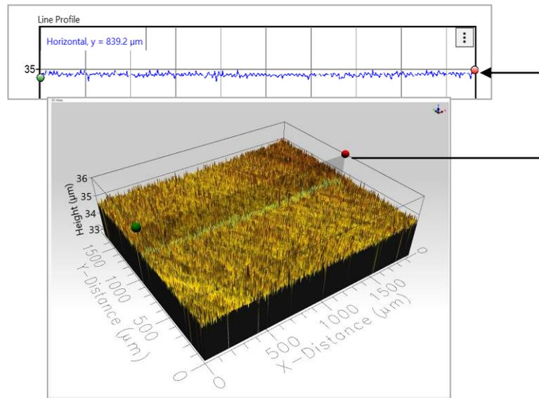
**Fig. 7** Surface scan of dry down milled specimen at 750 m/min and 0.009 mm/tooth. Surface roughness measured for this test were  $Ra = 0.083 \mu\text{m}$  and  $Sa = 0.110 \mu\text{m}$
