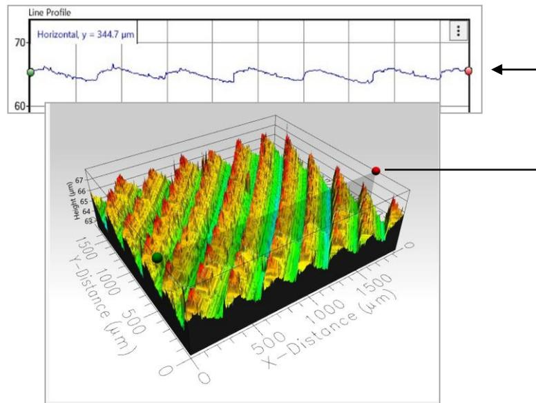
**Fig. 8** Surface scan of dry down milled specimen at 750 m/min and 0.15 mm/tooth. Surface roughness measured for this test were  $Ra = 0.647 \mu\text{m}$  and  $Sa = 0.754 \mu\text{m}$
