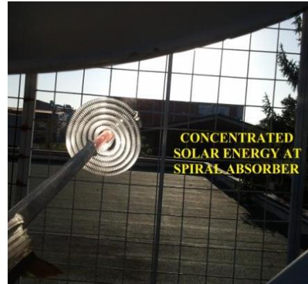
**Fig. 2** Concentration of solar radiation at the spiral absorber pipe
