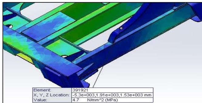
**Fig. 10** Stress value in the zone of strain gauge no. 16 - shell model
