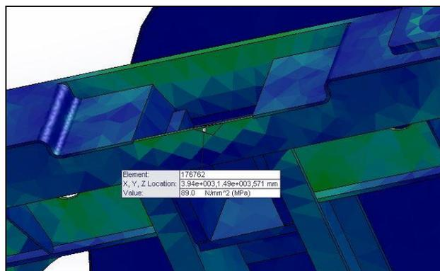
**Fig. 7** Stress value in the zone of strain gauge no. 2 - solids model
