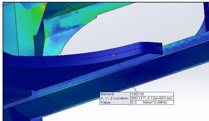
**Fig. 9** Stress value in the zone of strain gauge no. 16 - shell model
