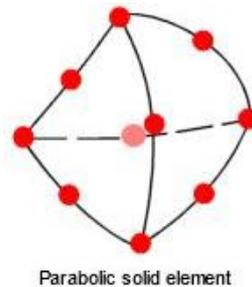
**Fig. 1** Finite element type 3D solid
