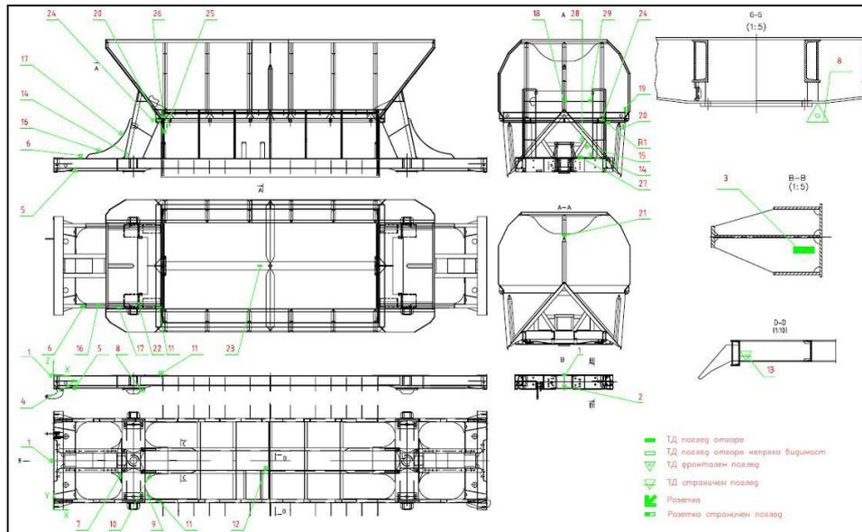
**Fig. 5** Plan of measuring points on wagon prototype
