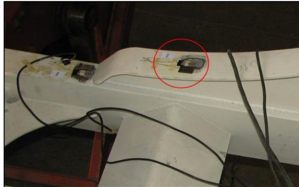
**Fig. 11** Strain gauge no. 16 – placement on wagon prototype during test
