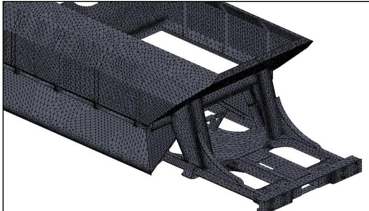
**Fig. 3** FEM model built up of finite elements type 3D solid
