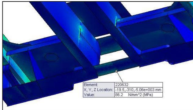
**Fig. 6** Stress value in the zone of strain gauge no. 2 - shell model
