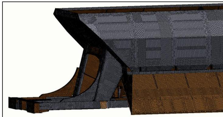
**Fig. 4** FEM model built up of finite elements type shell
