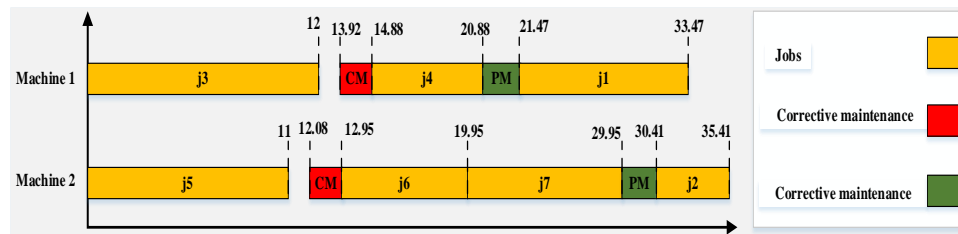
Fig. 1 Initial scheduling of the seven jobs on two parallel machines
