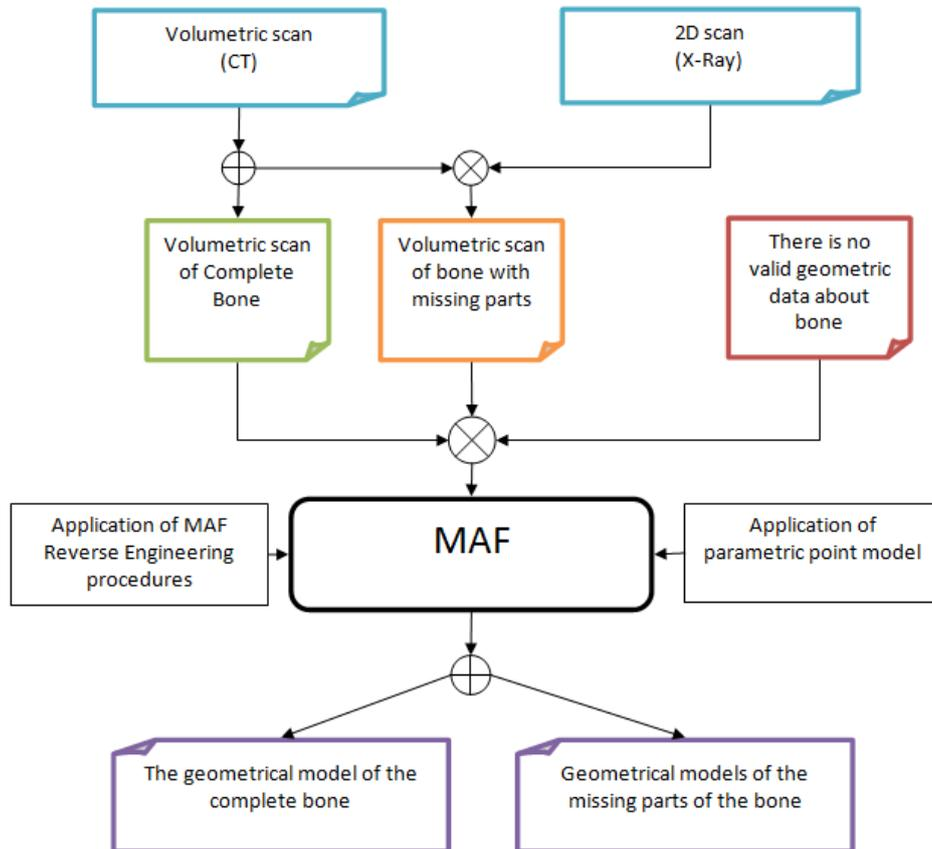
**Fig. 1** The components of MAF and its application
