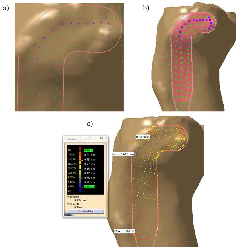
**Fig. 6** Definition of MIF-LTP contact surface with additional parametric points:
