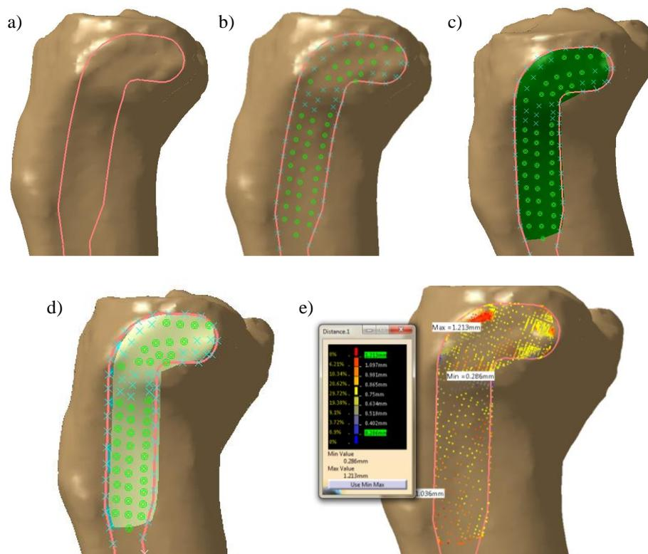
**Fig. 5** Definition of MIF-LTP contact surface with initial parametric points:
