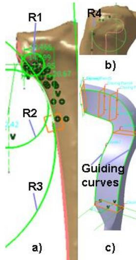
**Fig. 3** a, b) Constructed circles, c) MIF-LTP volume model
