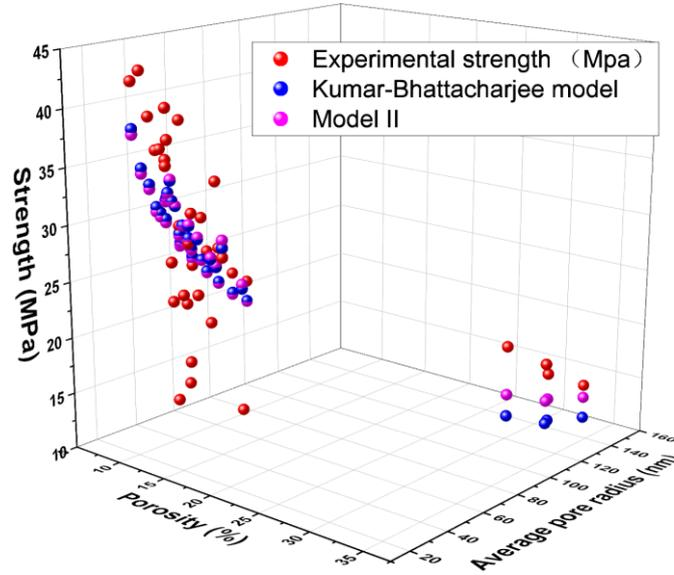
**Fig. 3** Comparison between the theoretical prediction of Eq. (43) and experimental data given in Ref. [43].
