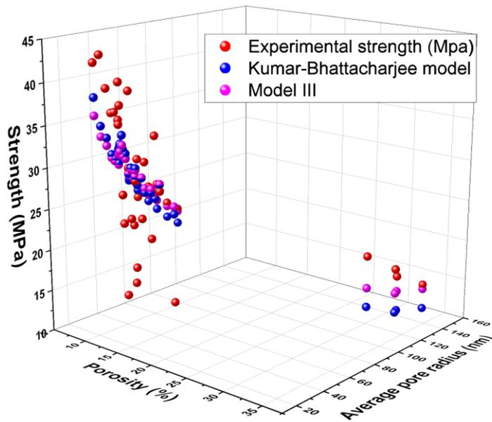
**Fig. 4** Comparison between the theoretical prediction of Eq. (47) and experimental data given in Ref. [43].
