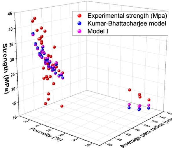
**Fig. 2** Comparison between the theoretical prediction of Eq. (38) and experimental data given in Ref. [43]
