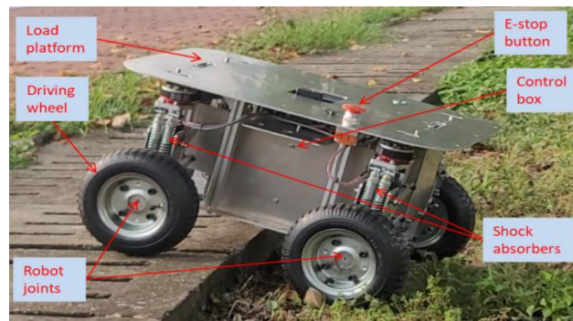
Fig. 15 Mobile robot test platform
