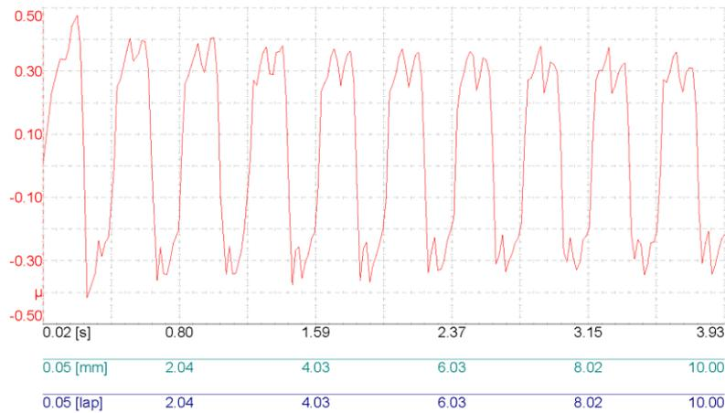
**Fig. 1** Dynamic friction coefficient for 10 cycles (test duration of 3.93s) (Sample 1, dry contact, 4 mm/s, 100mN)
